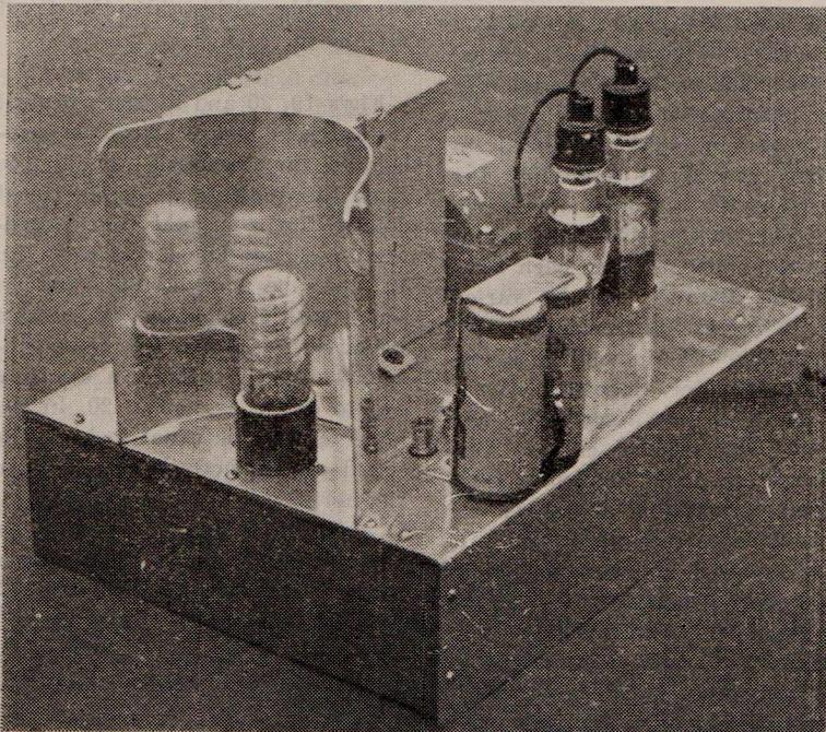
alongside the two high-voltage rectifiers. Next is the big reservoir condenser, with a cycle lamp battery on the other side. Behind the battery are two terminals for the contact leads.
