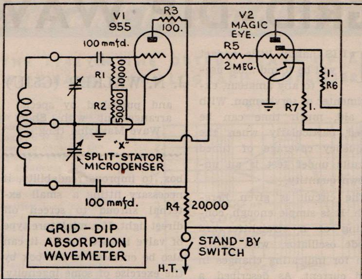
**GRID-DIP ABSORPTION WAVEMETER**
