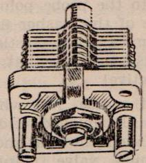
60 PF single section with provision for screwdriver adjustment instead of extended spindle. Mounting pillars supplied. Air gap .020ft.
