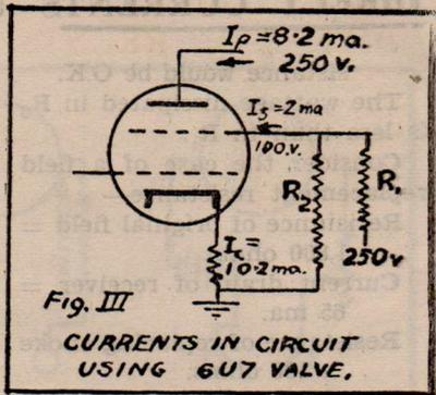
tual voltage at the plate of an ordinary resistance coupled amplifier. It is not difficult to arrive at this voltage if necessary by lifting the h.t. end of the plate resistance from its supply point and inserting a milliampmeter. Then, knowing the value of the plate resistance, and the current through it, the voltage drop through it may be calculated using rule (5) and this can be subtracted from the h.t. supply voltage.
