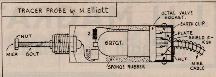
feed to both the 6J7G and the 6Q7GT is a definite must; 8mfd for the 6J7G and .5mfd for the 6Q7GT being quite sufficient.
