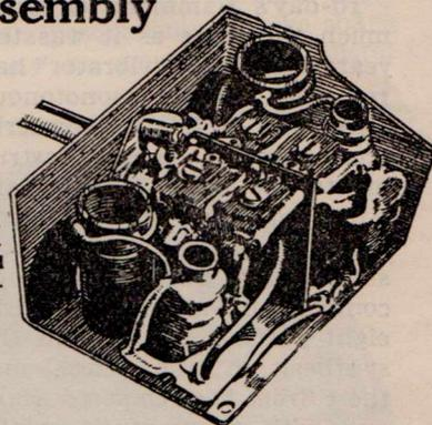
A dual-wave assembly, incorporating permeability tuned Aerial and Osc. Coils for B/C (550-1600 Kc) and S/W (7-23 Mc) Trimmers and Padder (fixed) condensers fitted. Iron Core adjustment
