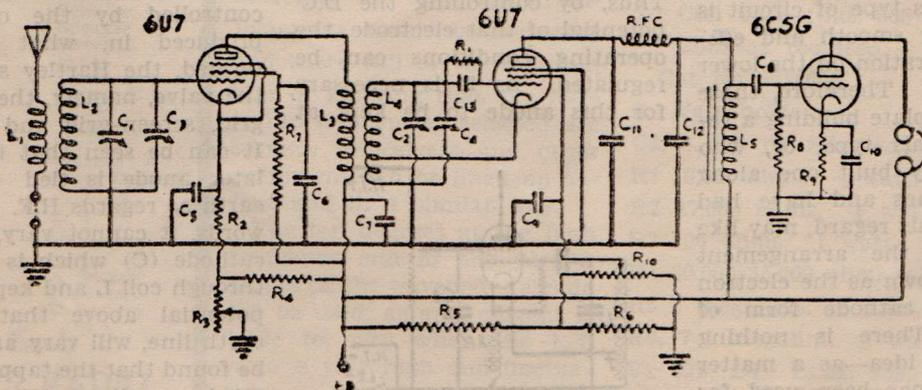
Fig. 4: Three-valve f.r.f. circuit.
