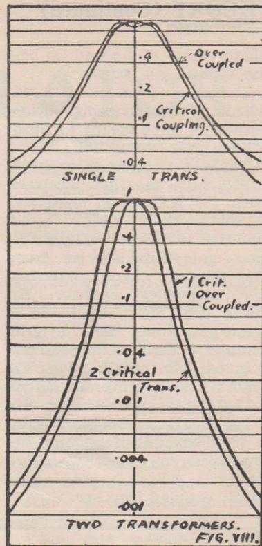
count the loading due to the plate resistance of the preceding valve. This plate resistance acts as a parallel resistance across the tuned circuit reducing the impedance, and therefore the Q of the coil. In practice the parallel plate resistance of a valve such as a 6SK7 with a plate resistance of 0.8 megohm will reduce the Q of an average coil from 130 to about 80. The input resistance which is usually in the order of several megohms has a much smaller effect.
