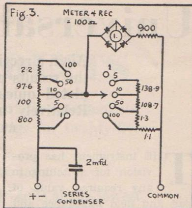
meter ranges were switched thus giving incorrect readings, in addition a series resistor would have to be included as the primary (in most cases) carries D.C. With the meter across the voice coil, however, the resistance of the meter is high compared to the low impedance of the voice coil on any of the three ranges.
