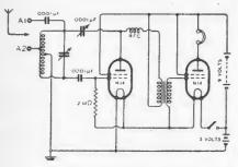
Suggested circuit diagram for two-valve headphone set to use a very low high-tension voltage. The valves are both of the "beam power" output type.
