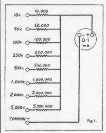
Schematic arrangement tor wide-range voltmeter.
