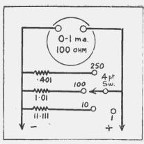
Arrangement for a four-range milliammeter, which is a handy instrument.
