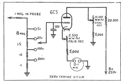
scale on the meter will determine the Circuit for a zero-centre vacuum tube voltmeter for a.c. operation. Below: Circuit for a V.T.Y.M. suitable for battery operation.
