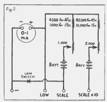
Diagram for a three-range Ohmeter of infinite value to the serviceman.
