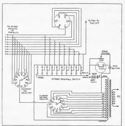
Circuit of the versatile valve tester
