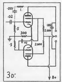
The circuit for use with beam power valves.
