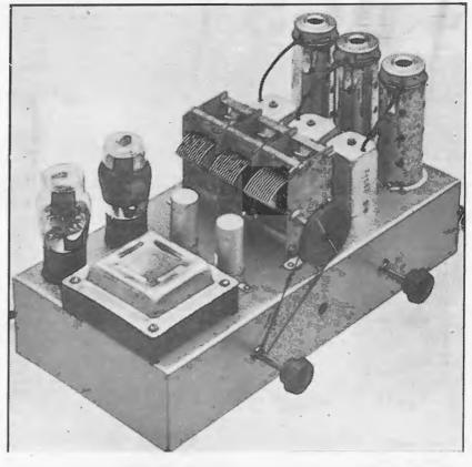
A general view of the finished chassis, Any desired style of dlal can be substituted.
