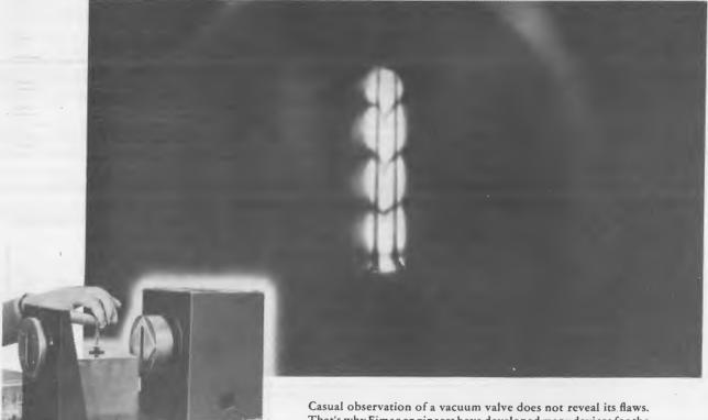
Observation of the stress points on glass bead seals around vacuum valves leads is made with this device. Close-up photo above shows the actual view of a faulty lead. Note the change in polarized light creating distorted shadows which show up stress and strain in beads. Such strain sometimes occurs where metal and glass are sealed together.
