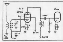
Diagram showing use of untuned r.f. stage.
