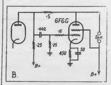
Circuit of normal audio end, but with changed component values to give improved overload characteristics.
