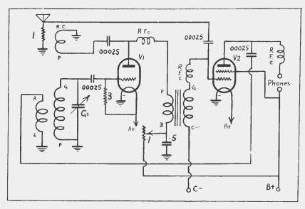
The output pentode of almos@ any battery set can be used to amplify the signal before it is applied to the aerial coil, as shown in this diagram.
