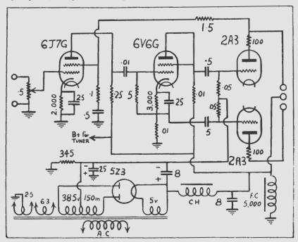
Circuit of the audio end and the power supply. Two resistors are required to: make up the 345 ohm bias resistor, as detailed in the article.
