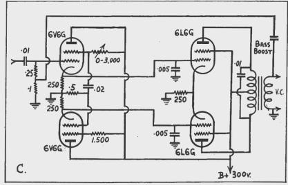
Circuit for Class AB2 operation without the use of a special input transformer.
