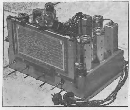
A photograph of the tuner and amplifier. The power unit is built on to the speaker base as shown in the October issue.
