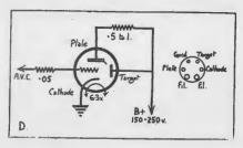
Diagram of the connections for a cathode-ray tuning indicator (magic eye).
