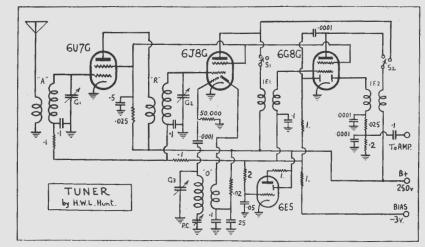
Schematic diagram of the tuner portion of the super-quality dual-wave receiver.
