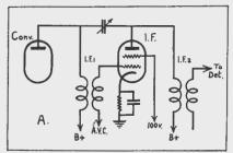
Diagram showing how to increase the range of a superhet by fitting reaction to the inter-mediate stage.
