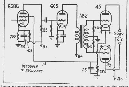
Circuit for automatic volume expansion, taking the screen voltage from the bias resistor of the output valves.
