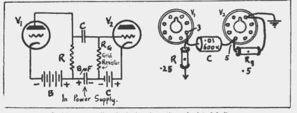
Resistance coupling in both schematic and pictorial diagrams
