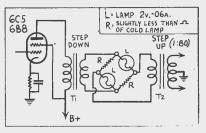
A pilot light bridge arrangement for automatic volume expansion.
