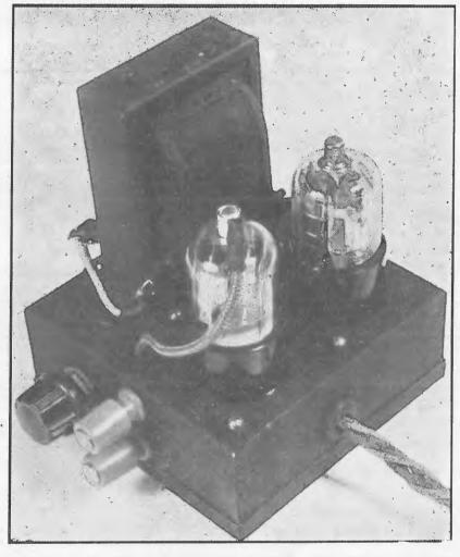
A photograph of the unique little battery-operated amplifier, which uses only two output pentodes.
