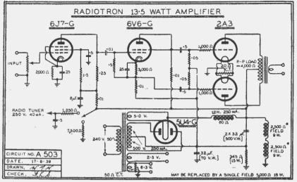
Circuit of the Radiotron circuit A503, which was originally released in 1939. Since that time it has proved itself to be a particularly effective and handy circuit.
