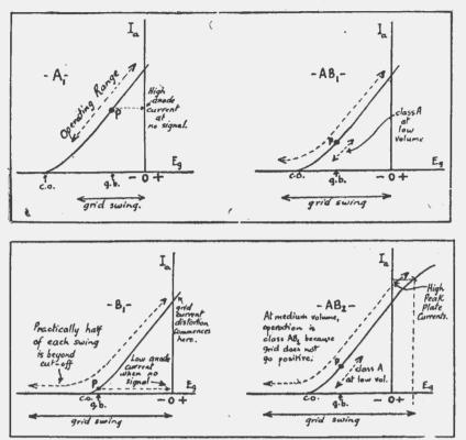
Typical grid-plate curves of output valves to illustrate the different classes of operation.
