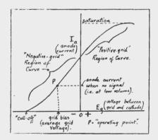
positive. If the signal voltage exceeds the grid bias voltage, then the grid will become positive at one end of the swing and because a positive body attracts electrons, grid current will flow at these times. To indicate that grid current flows, the figure 2 is used. Note:-In the case of class AB AB1 for medium-sized signals, and cycles.
