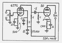
suggested circuit, with a large power triode driven by a pentode first-audio valve.
