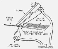
Fig. 2. Suggestions for an improvised electric welder for joining the power leads to the leading-out wires of the heater element. The accumulator leads must be of heavy cable, as short as possible.
