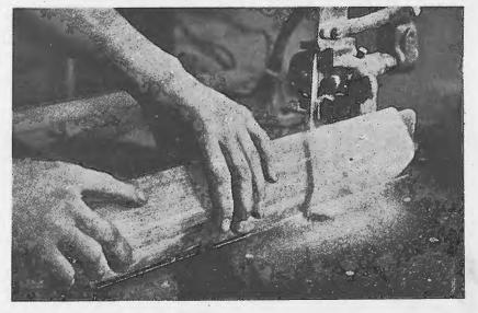
Sawing up a big block of rochelle salt to make crystals for the control of transmitter oscillators.
