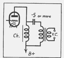
Schematic to show shunt-feed arrangement to improve efficiency of the output transformer. bias, we can say that we need the feeding for the output transformer, valves needing high bias voltages, as preceding value to be capable of de- passing the high tension current the ordinary by-pass electrolytics of livering a signal voltage of at least through a heavy choke, such as a big 25 mfd. 25 or 40 volt rating cannot this amount.
