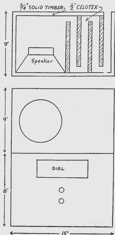
Suggested construction of an acoustic labyrinth for use with the direct-coupler or any other receiver with good tone.
