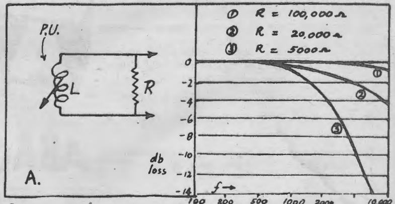
Attenuation of "Highs" by Resistor Shunt.
