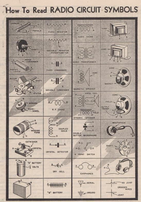
Once you understand meanings of schematic symbols pictured in two vertical center columns above, radio circuit diagrams will no longer be a mystery. Pictorial sketches are shown at right or left of each symbol, with letters to show proper conmections. Remember that short bar on battery symbol is always negative. Use terminals A and B for variable resistor; slt three for potentiometer. B on potentiometer is always movable contact. Parallel lines always indicate iron core.
