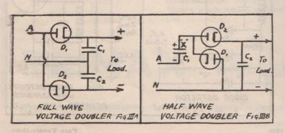
same in each case, the utilization of both halves of the sine wave to get double the voltage.
