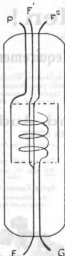
Fig. 2—The Valve—Showing Arrangement of Elements.
