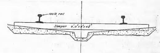
Showing the arrangement of the sleepers underground to provide for easy riding and to enable the subways to be hosed down and dust washed away.
