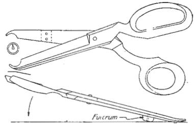
An Old Pair of Scissors Used in Making a Thumb-Tack Puller
