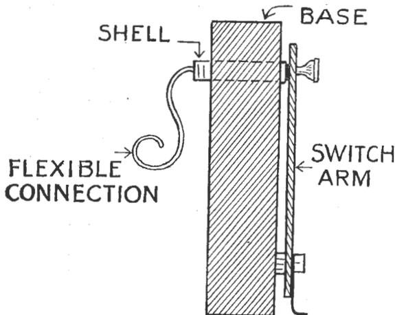
pushing in the shell. Connections may be soldered into the shell, the bottom of which makes contact with the switch.
