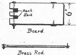
made running lengthways. The pieces of metal between the saw-cuts are then broken off, leaving two pieces projecting down. These are flattened, and a  $\frac{1}{4}$ -inch hole drilled near the end.
