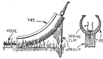
An Old Automobile Tire Makes Support for Holding Hose in Position for Sprinkling Lawn
