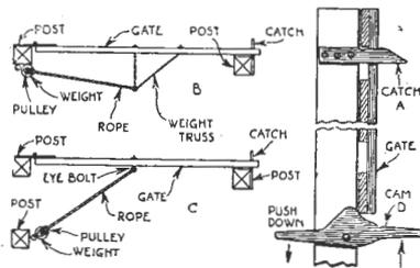
Release for a Gate Latch Operated by a Foot Lever
