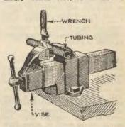
monkey wrench in the manner illustrated. Adjust the wrench jaws until the work will rest only on the edges of the jaws; clamp the wrench and work in the vise in the position shown, and the stock will be held as securely as in a pipe vise.—"Popular Mechanics."
