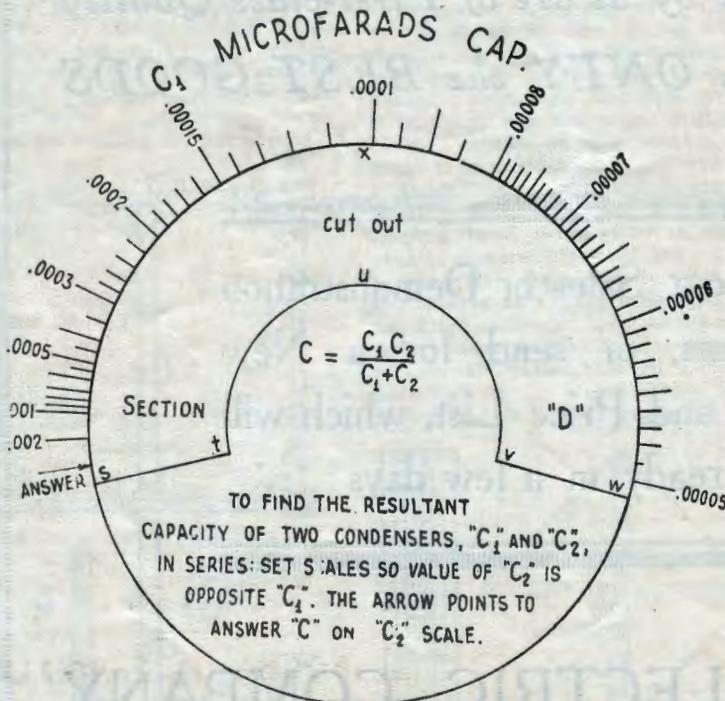
densers are connected in series the resulting capacity is always less than that of either condenser alone, the exact value being ordinarily determined with the formula appearing at the centre of the scale section C. This slide rule gives the answer to this formula directly.
