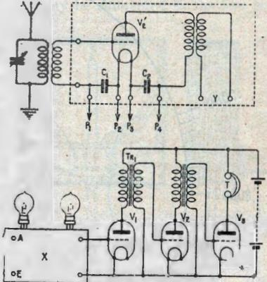
V1, the subsequent L.F. valves being designated V2 and V3, the plate circuit of the last valve including the telephone receivers T. Between the valves V1 and V2, and between V2 and V3 are the usual L.F. interval transformers. This or any
