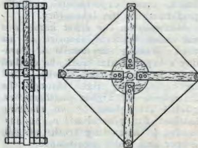
cessed bearing block secured to the inside of the top of the frame as shown. (See also sectional view G.) This arrangement provides a simple means of swivelling the frame on its own axis. The lower end of the broom handle is secured to any suitable base.
