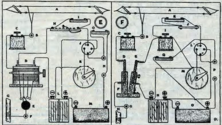
A. Aerial; B. Aerial Terminal; C. .0005 Mfd. variable condenser; D. Vario-coupler; E. Multiple switch; F. Earth Terminal; G. Earth; H. Variable grid leak; I. Grid condenser; J. Valve; K. Filament rheostat; L. Accumulator or low tension battery; M. High tension battery; N. Phone terminals; O. Phone condenser.
