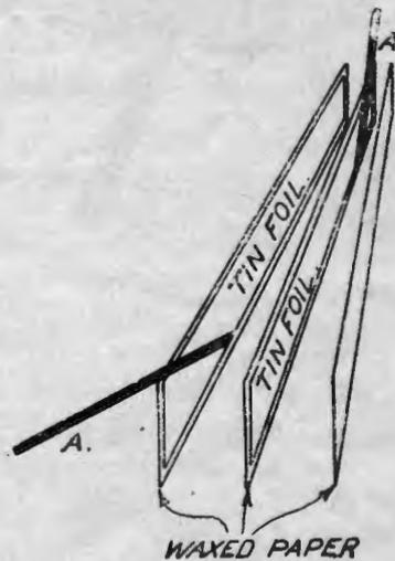
cut the tin foil into two long strips the size required, and rolling them up together using as the dielectric good quality paper previously soaked in paraffin wax. The strips of paper should be  $\frac{1}{2}$  inch larger all round than the sheets of foil. Be-
