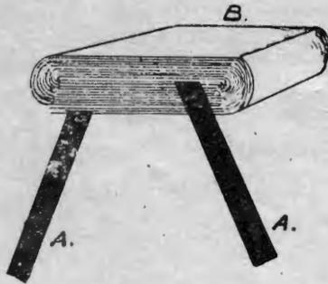
bolt them to each end, firmly clamping the copper foil strips beneath them as shown at D. Melted paraffin wax poured round the edges of the condenser will make it damp proof.
