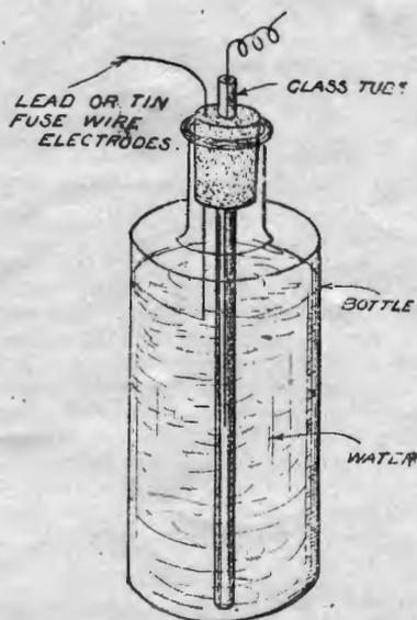
Fig. 8.—The completed resistance.
