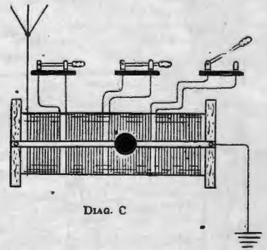
An adjustment of the switch arm will, of course, necessitate a corresponding adjustment of the slider, since each section of the winding represents a self-contained coil connected to a common earth. The setting shown in the diagram indicates that only the first section is in circuit. This section could be conveniently arranged to just cover the broadcasting wave lengths. By moving the switch arm to the next stud on the right, the aerial lead-in is connected from
