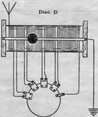
Diagram D shows how a radial dead-end switch may be fitted to a large cylindrical inductance coil.
