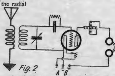
Showing the Connections of the Set When Used With an Aerial and Ground. An External Variometer Is Included, to Obtain Regeneration
