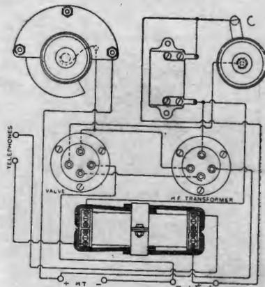
Fig. 6. Connections of the testing instrument.
