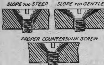
—Illustrating correct and incorrect countersinks
