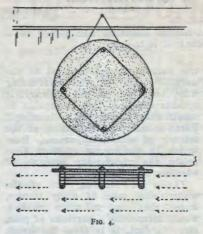
a flat box-like frame, provided at each corner with rubber or ebonite angle pieces H, having small nicks cut as shown to form pacing beds for the wire. Thin sheet ebonite may be bent in this way if it is heated. Each side should be 3 ft. 6 in. long, and the width will, of course, depend on the number of turns it is proposed to wind on.
