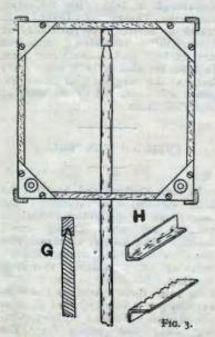
wire and providing a correspondingly extra number of binding posts, 14 turns tuning fairly accurately on 900 metres, 16 turns on 1,080 metres (Hagne), 23 turns on 1,600 metres, and 34 turns on 2,500 metres. As pointed out, the wire is wound on in spiral formation.
