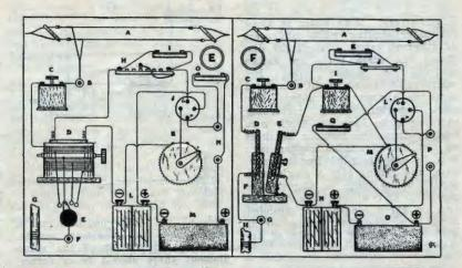
A. Aerial; B. Aerial Terminal; C. 3005 Mfd. variable condenser; D. Vario-coupler; E. Multiple switch; F. Earth Terminal; G. Earth; H. Variable grid leak; I. Grid condenser; J. Valve; K. Filament rheostat; L. Accumulator or low tension battery; M. High tension battery; N. 'Phone terminals; O. 'Phone condenser.
