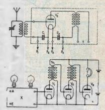
V1, the subsequent L.F. valves being designated V2 and V3, the plate circuit of the last valve including the telephone receivers T. Between the valves V1 and V2, and between V2 and V3 are the usual L.F. intervalve transformers. This or any
