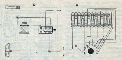
made all the difference between a dead silence and maximum results. To every adjustment of the valve filament there should be a corresponding adjustment to the plate current. Many enthusiasts overlook this important fact. But it will soon be discovered that the most critical thing to contend with is the value of the grid leak and condenser.
