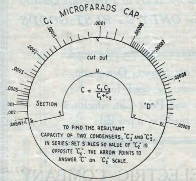
densers are connected in series the resulting capacity is always less than that of either condenser alone, the exact value being ordinarily determined with the formula appearing at the centre of the scale section This slide rule gives the answer to this formula directly.
