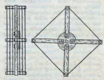
cessed bearing block secured to the inside of the top of the frame as shown. (See also sectional view G.) This arrangement provides a simple means of swivelling the frame on its own axis. The lower end of the broom handle is secured to any suitable base.
