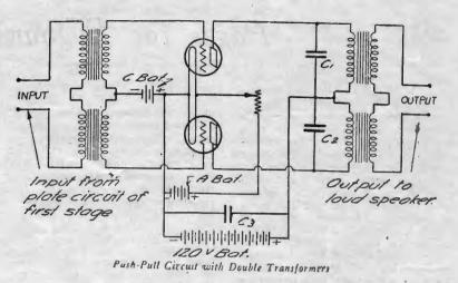
amplification may, be secured by shunting the respective secondaries and primaries of single transformers with a resistance whose midpoint is tapped.
