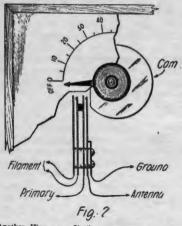
Another View of a Similan Arrangement, Which Can Be Attached Directly to the Shaft of the Tuning Variable Condenser
