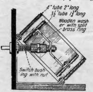
Pig 1 Constructional Details of the 360-degree Variometar The Two Brushes Are Attached Direquip to the Front Panel and Make Contact With the Split Ring on the Wooden Washer the windings of the coils are equal. As the rotor is turned through 180 degrees, the inductance increases, until it equals the sum of the inductances of the two coils, viz., the
