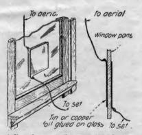
A Clever Stunt in the Form of an Aerial Lead-In The Marial Shaets to. Which the Wires Arc Connected Act as a Condenser
