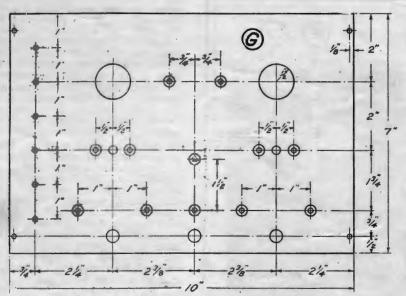
HOW TO DRILL AND CUT THE PANEL FIGURE 4: This diagram gives the correct locations for the holes for the instruments and the binding posts. The holes outlined here with a double circle should be connersunk; the rest of the holes are straight drill holes.
