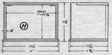
THE DIMENSIONS OF THE CABINET This may be made by the builder himself, or the plan may be turned over to a cabinet maker The woodwork may be done in any kind of hardwood that conforms to the owner's taste.
