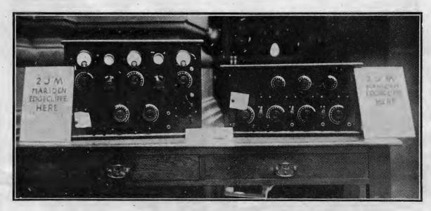
5 valve Neutrodyne and 10 Watt Transmitter. Mr. R. C. Marsden's Exhibits
