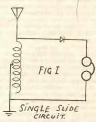
If a single slide (Fig. 1) crystal receiver is being used and the interference is only slight, probably another slider will fix matters up.
