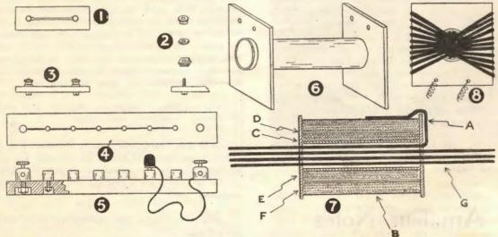
and drill two holes for the terminals about 1 in. apart.. Cut a small groove along the surface of the ebonite between the two holes and widen the groove at each end where it merges into the holes. (See Fig. 1).
