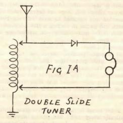
The circuit is shown in Fig. 1A, and as will be seen is quite a simple matter to instal, nothing being required except a slider and screws for mounting it. If the interference is very pronounced, a two-circuit tuner or loose coupler, as it
