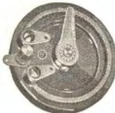
Resistance element is machine wound, giving even spacing of wire, and is securely held in deep recess in bakelite body. Phosphor bronze contact finger, giving smooth operation over entire range.
