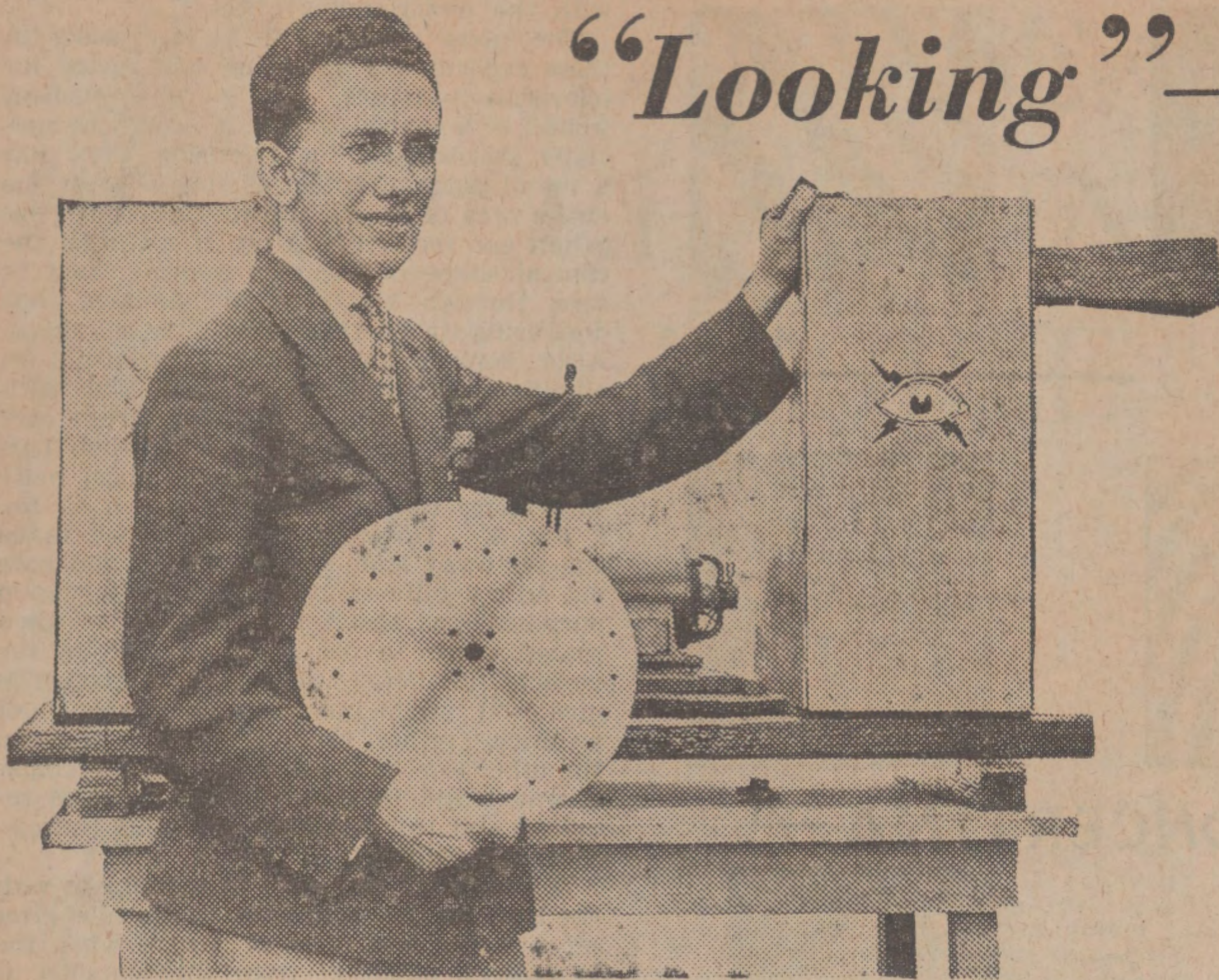
Mr. W. G. Nichols, with the apparatus. He is holding the scanning disc in his hand.
