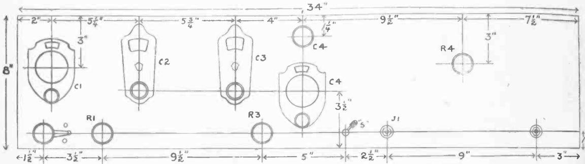
The template supplied with the dial shows exactly where drilling must be done to cut away the aperture for the indicator dial, and the knob drive at the bottom. Do not worry about insulating the frame of the dials from the aluminium, as the condenser is mounted directly on the frame by the rotor alone, and the whole is earthed with the A positive and B negative.
