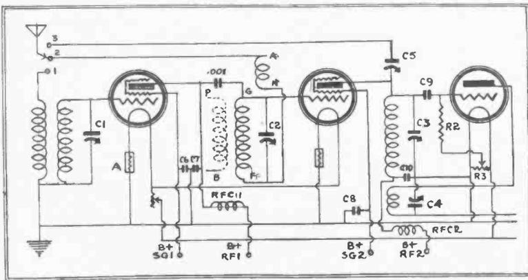
Theoretical Circuit Diagram, illustrating alternative method of coupling first and second RF stages. The primary coil in this case is not used. Compare
