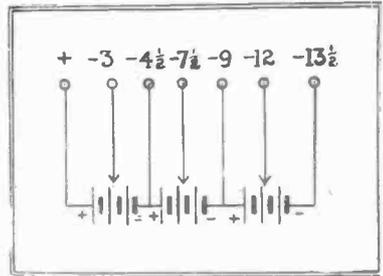
**E.K. Queensland, asks for a diagram showing how to connect up two "C" batteries in order to obtain various negative tappings.**
