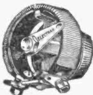
THE resistance element is the finest material known. Its value is guaranteed within 5 per cent. High-grade Bakelite insulation. Metallic bearings. Overstressed contact arm of phosphor bronze. Milled shaft with square hole in contact arm prevents shaft or knob from turning without moving contact arm.
