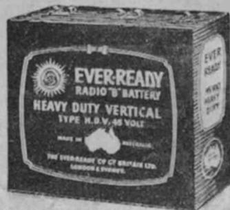
The EVER-READY HEAVY-DUTY 45 Volt "B" Battery. 30 large cells in hermetically sealed moisture-proof containers with positive tapings at 18, 24, 30, 45 volts.
