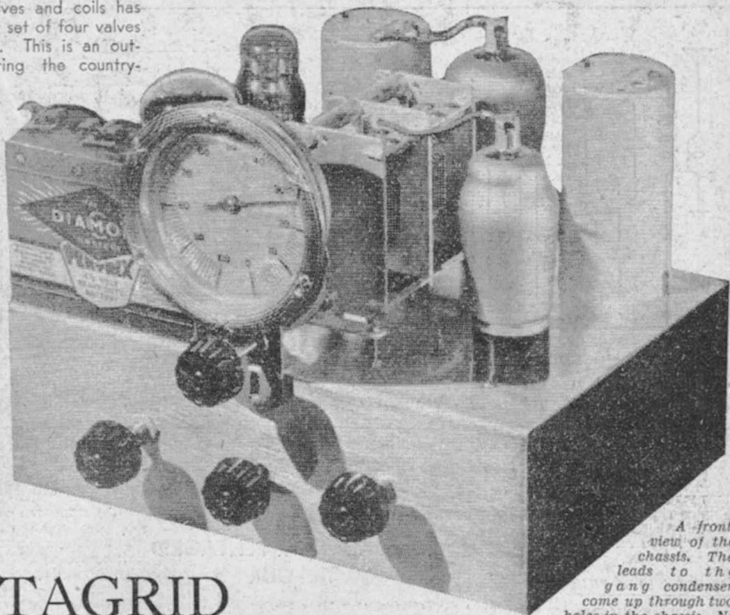
A front view of the chassis. The leads to the gang condenser come up through two holes in the chassis. No valve cans are required.
