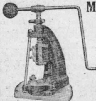
Bench Screw Press (Quick-acting, Fine Adjustments).
