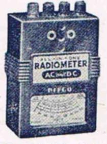
Pifco A.C.-D.C. Radiometer, 32/6. Reads everything in radio, for testing valves or sets. Reads 0 to 30 m/a., 0 to 6 or to 240 volts.
