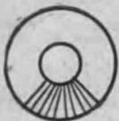
When the "Magic Eye" is as shown it indicates that the reception is either from a weak station, or if reception is coming from a station nearby your radio set is not tuned-in correctly.
