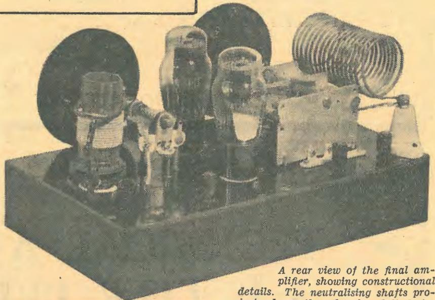
A rear view of the final amplifier, showing constructional details. The neutralising shafts project above the chassis, slotted for adjustment.
