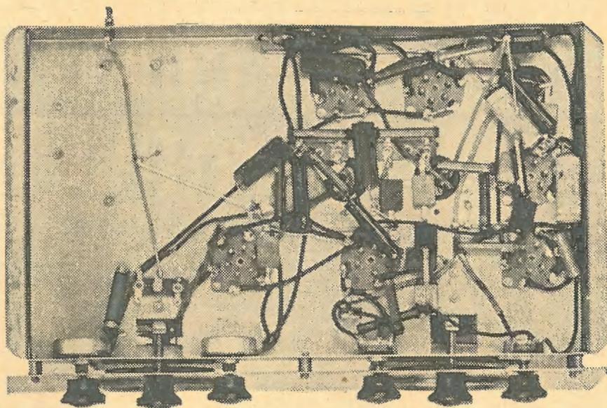
A sub-base view of the set. Note the free use of mica condensers, and the short leads.
