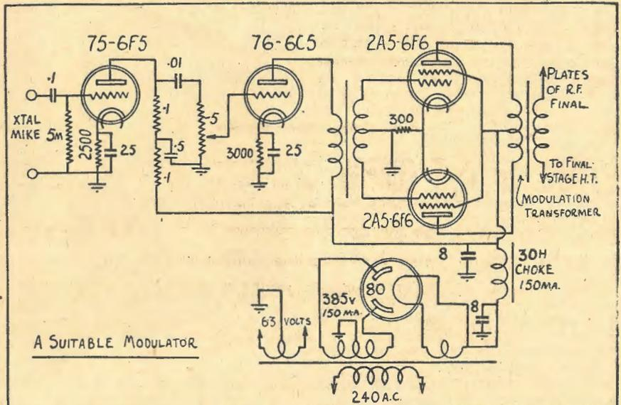
Here is the circuit of a suitable modulator which may be used with the transmitter for 'phone operation. It is merely a straightforward, high-gain amplifier.
