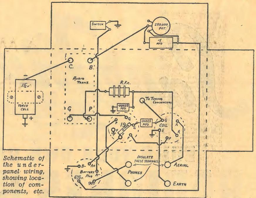
Schematic of the under-panel wiring, showing location of components, etc.
