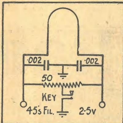
Showing the position of the key in the final stage, when the transmitter is to be used for C.W. work.
