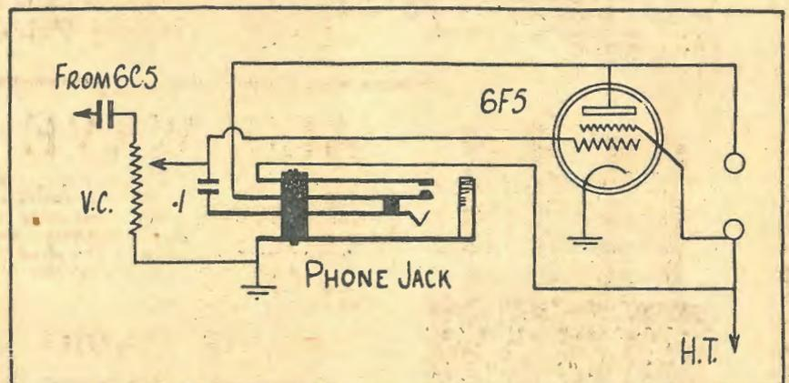
The circuit showing how to use headphones with the set. The jack need not be insulated from the panel. When the plug is inserted, the speaker is silenced, but the volume control still operates.
