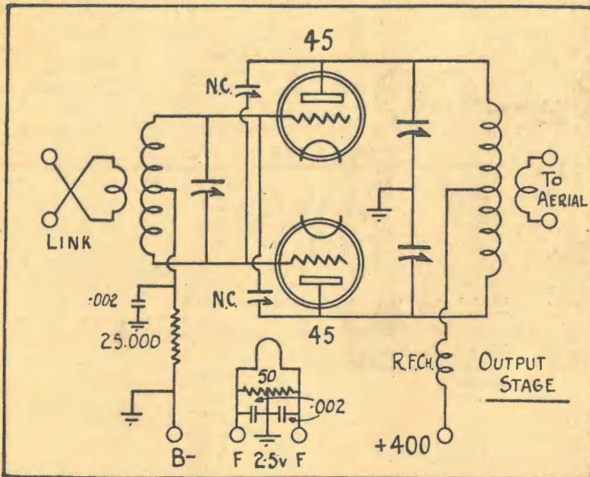
The circuit of the push-pull final amplifier. In C.W. work the key is inserted between the filament centre top and earth. A separate diagram shows just where this should be placed.
