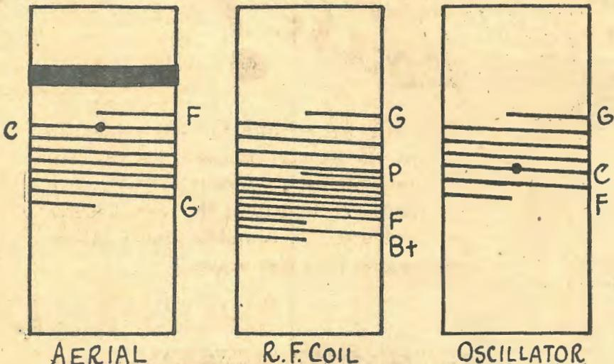
This drawing shows the relative connections for the coils. The black band on the aerial coil represents the aerial coil itself. Connections to it are brought out to two insulated terminals at the rear of the chassis for doublet connection. We advise such an aerial. If a plain aerial is used, the end of the coil nearest F of the grid coil is earthed. Note the partial interwinding of the R.F. plate coil. The dot opposite "C" indicates the tapping.
