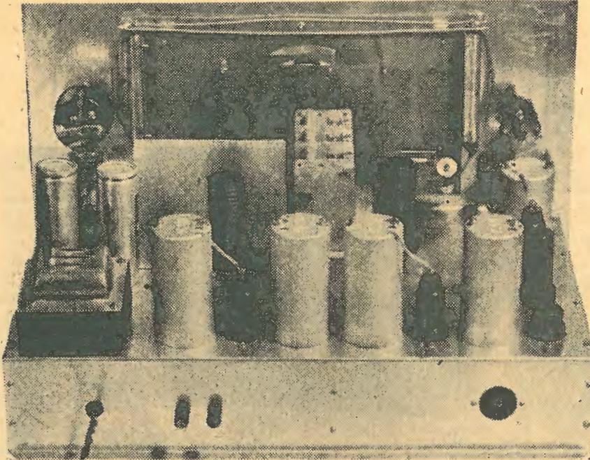
The set from the rear. Many constructional points are visible here, notably the I.F. channel, and screen between the aerial and R.F. coils.
