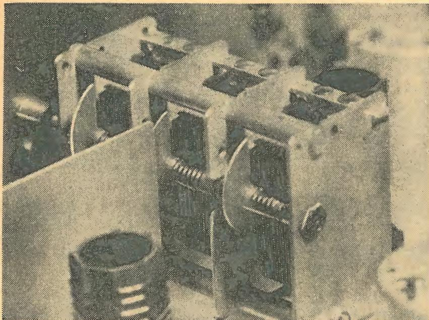
A close-up of the tuning gang, showing the cut-down plates of the tuning condenser. It is only necessary to do this for amateur work. As a general short-wave set, use a regular 3-gang .00015 capacity (approx.) gang condenser.
