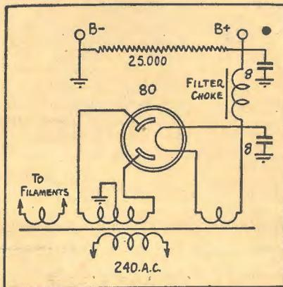
Circuit of a typical power supply suitable for this transmitter. Standard 385 volt 150 mill. transformers are used.
