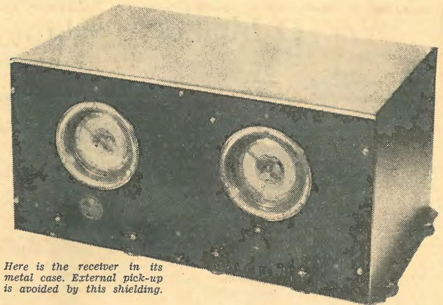
Here is the receiver in its metal case. External pick-up is avoided by this shielding.
