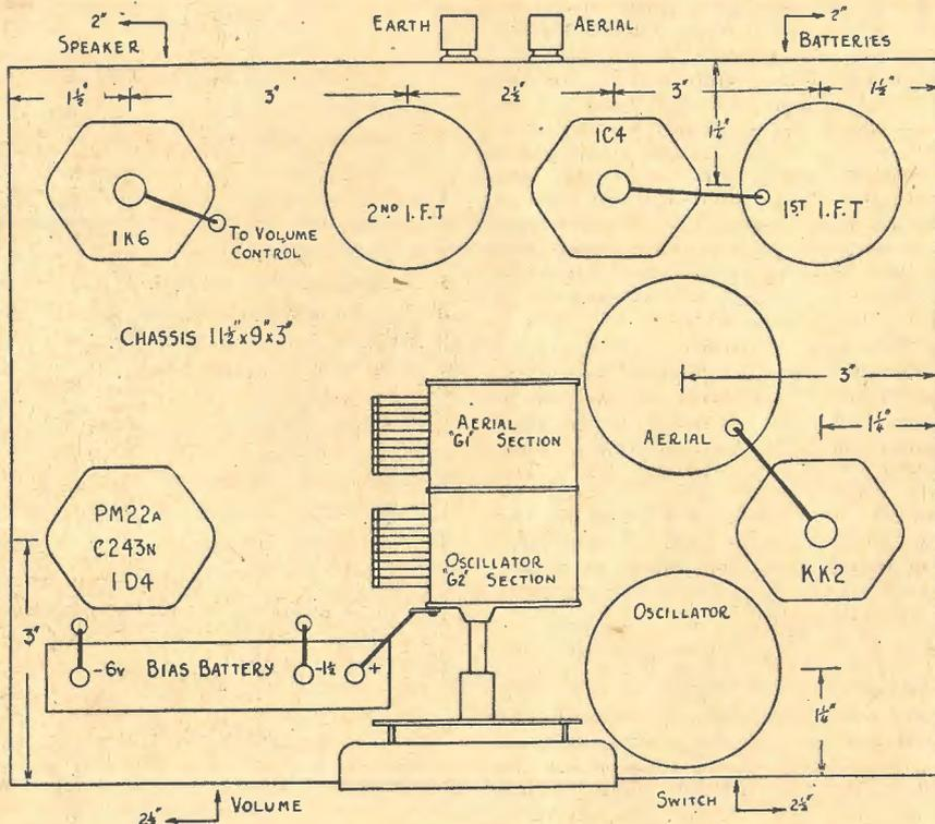
This drawing gives an idea of how the chassis is laid out. If possible, always check up with actual components before finally drilling the chassis.
