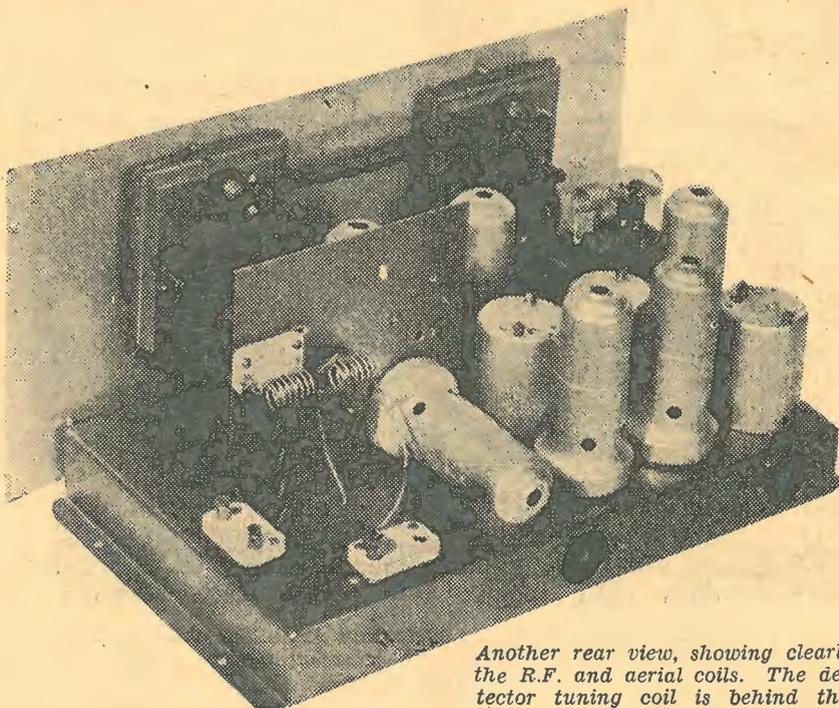
Another rear view, showing clearly the R.F. and aerial coils. The detector tuning coil is behind the shield.
