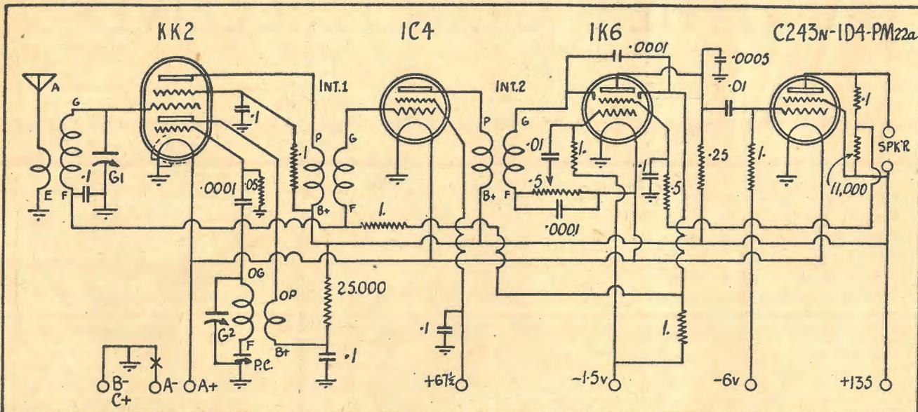
The circuit of the receiver. It is often a good idea to include a .5 mfd. tubular condenser from the 135 volts high tension to earth. The A.V.C. line is here shown with a bias of 1.5 volts. See text.
