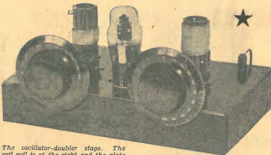
*The oscillator-doubler stage. The grid coil is at the right and the plate at the left. The base has a bakelite top and wooden sides.*
