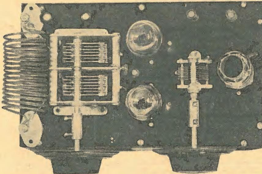
This plan-view of the final amplifier gives an excellent idea of the layout. The neutralising condensers are mounted under the base in front of each valve on the grid coil side.
