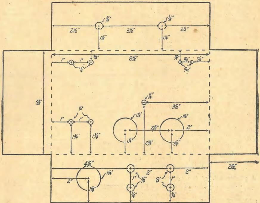
A diagram to show the actual drilling of the original base. The mounting holes for the gang and the valve sockets have not been shown, as these will vary with individual components.
