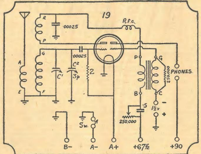
The circuit diagram. C1 is the main tuning condenser, an ordinary single-gang of .00035, .000385, or .0005 mfd. capacity.
