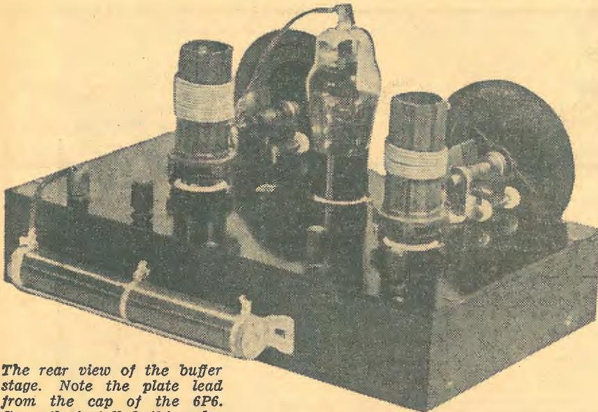
The rear view of the buffer stage. Note the plate lead from the cap of the 6P6. Correctly installed, this valve needs no neutralising.
