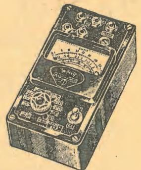
**TRIPLITT D.C. MOVING COIL INSTRUMENTS** are of the D'Arsonval type with an extra light moving coil and reinforced strong parts. Sapphire jewel bearings. Accuracy within 2%. Permanent magnets. Supplied in sizes from 2½ in. diam. to 5½ in. diam. (flange). Model 421 (at left) 4½ in. x 4 in.
