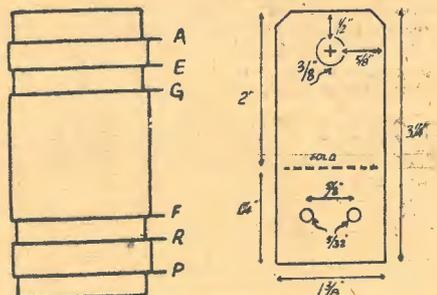
Left: Diagram showing coil connections. Right: The mounting strip for the trimmer condenser.
