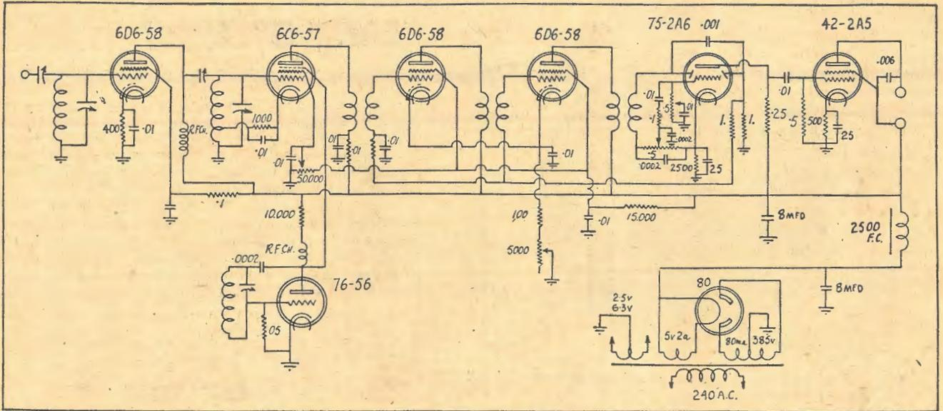
Here is the circuit of the receiver. Note that either 2.5 volt or 6.3 volt valves can be used. Metal types should also be suitable, but present no advantages. The aerial may be capacitively or inductively coupled.
