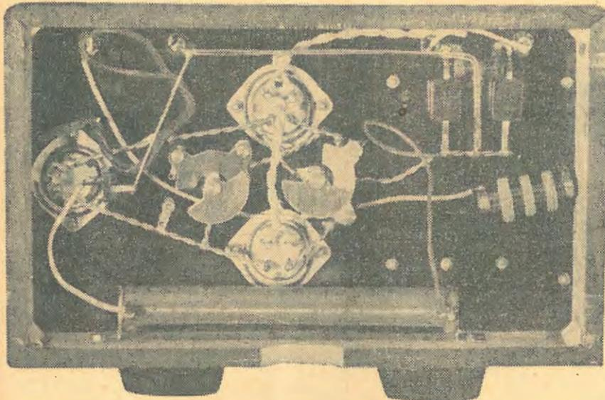
A view taken from beneath the chassis of the power amplifier, showing the neutralising condensers and valve sockets. The filament bypasses are necessary in this stage.
