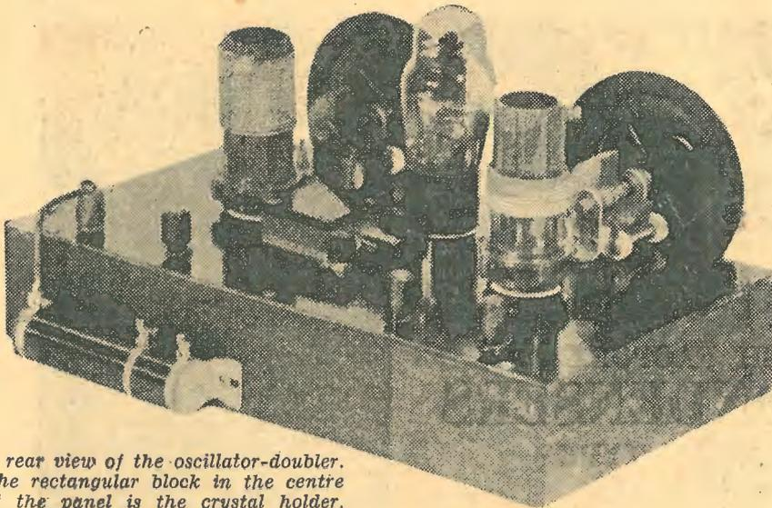
A rear view of the oscillator-doubler. The rectangular block in the centre of the panel is the crystal holder. Note the Steatite coil sockets and Isolantite condensers.
