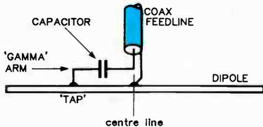
Figure 5. General form of the 'gamma match'. The tap provides an impedance match to the coaxial cable, but the gamma arm introduces a small inductance. This is tuned-out by the capacitor in series.
