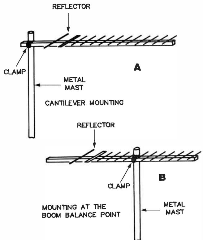
Figure 9. Horizontal polarisation mounting arrangements — (a) shows cantilever mounting, while (b) shows mounting at the boom balance point. In both instances, a metal mast may be used.
