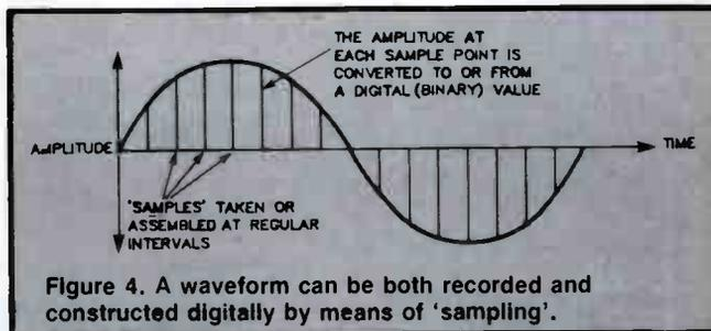
Figure 4. A waveform can be both recorded and constructed digitally by means of 'sampling'.
