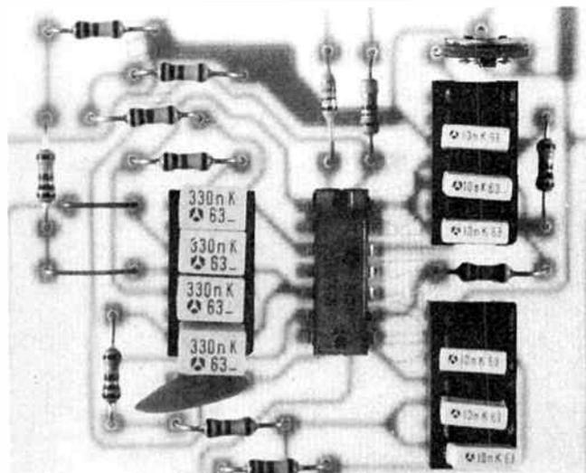
The active crossover has a number of extremely significant advantages over the more common passive designs. Firstly, active crossovers can be designed with much steeper slopes and the frequency response characteristics are much more predictable since there is no interaction between the filter and the highly non-linear load represented by the driver. The resulting well defined passbands help to decrease intermodulation distortion and optimise the frequency response performance.
