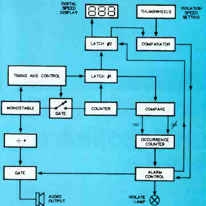
displays it, etc. There is provision for sounding an alarm if a preset value is exceeded and to latch the number in the counter if desired when this condition occurs.
