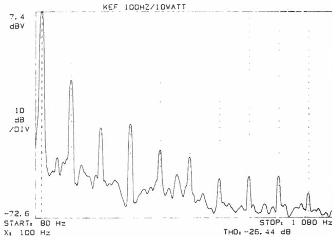
Figure 13. THD of the C10 at 100 Hz and 10 watts (always a critical parameter with bookshelf speakers) is a creditable -26.44 dB.
