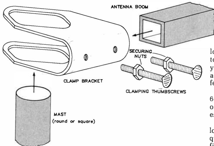
**Figure 10.** The beam is secured to the mast with this specially-designed U-clamp. Note that either round or square-section mast may be employed.
