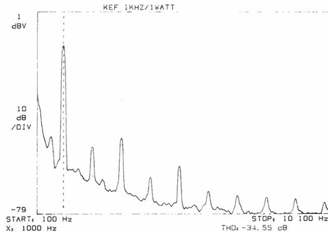
Figure 14. THD of the C10 at 1 kHz and 1 watt is excellent at a little better than -34 dB.
