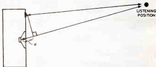
Figure 1. With conventional speaker cabinets the difference in the distances of the drivers to the listening position results in destructive interference of the sound waves producing a dip in the loudspeaker's frequency response where  $d = \frac{1}{2}$  wavelength. This is particularly a problem around the crossover frequencies.
