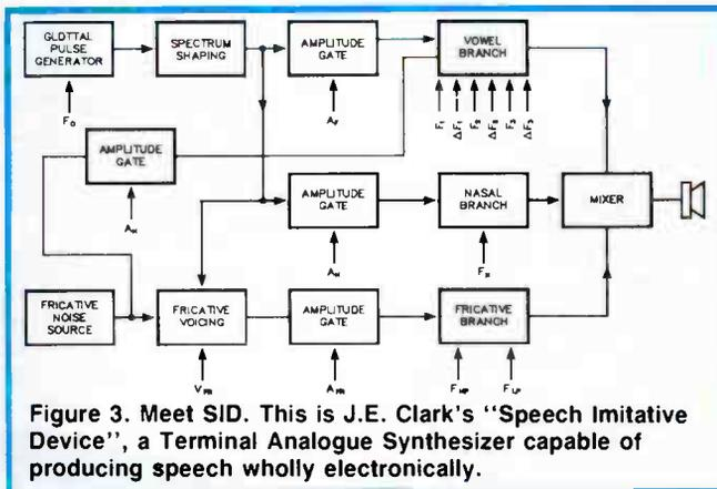
Figure 3. Meet SID. This is J.E. Clark's "Speech Imitative Device", a Terminal Analogue Synthesizer capable of producing speech wholly electronically.
