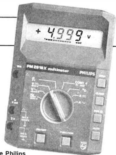
The Philips Series 18 DMMs feature 4.5-digit LCD readouts and a variety of sophisticated and useful functions — plus the unique option of automatic display backlighting under dim light conditions. The 2518 is the 'junior burger', the 2618 the 'quarter pounder' and the 2718 the 'big mac'! Range selection is by a single rotary switch, function selection by pushbuttons. Note the test leads and probes insert in the left hand side.
