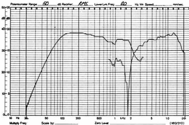
Figure 9. Near field responses of the two drivers in the C10 speaker.
