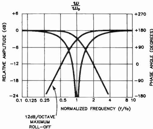
N.B: An infinitely deep hole results in the frequency response at the crossover point.  $V_{OUTH}(S)$  and  $V_{OUTL}(S)$  are 180° out of phase. To correct this the phase of one of the drivers is reversed resulting in the following frequency response.
