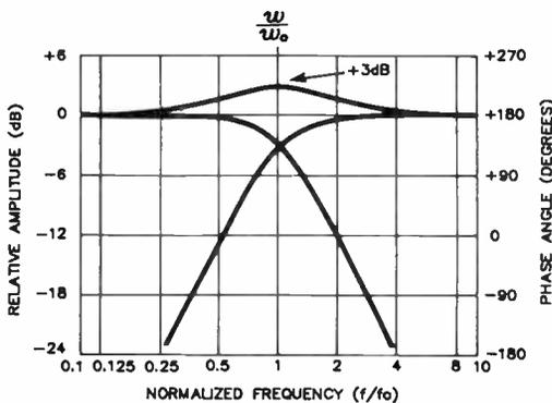
Figure 2, the second-order crossover results. A quick glance at the transfer functions and resulting overall frequency response shows that this crossover is entirely unsuitable for use in loudspeakers. The overall frequency response shows an infinitely deep hole at the crossover point which is caused by phase cancellation between the outputs of the filter sections.
