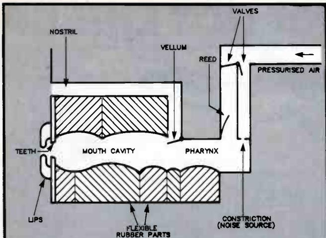
Figure 1. The mechanical vocal tract model proposed by Reisz in 1937. It was supposed to be 'played' by operating the valves with levers varying the flexible cavity parts.
