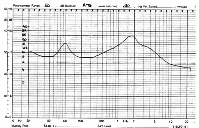
Figure 12. Impedance versus frequency response of the C10 speaker.
