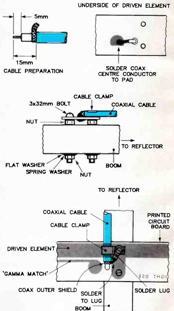
Figure 7. How the feedline connection is terminated and the driven element assembled.
