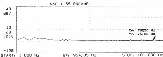
Figure 4. NAD 1155 preamp frequency response.
