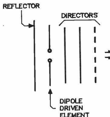
Figure 3. General form of the Yagi antenna. A halfwave dipole is the driven element. The reflector is a few per cent longer, directors a few per cent shorter. The reflector is spaced about one-fifth to one-quarter wavelength behind the driven element. The directors are spaced between about one-tenth and one-fifth wavelength apart.
