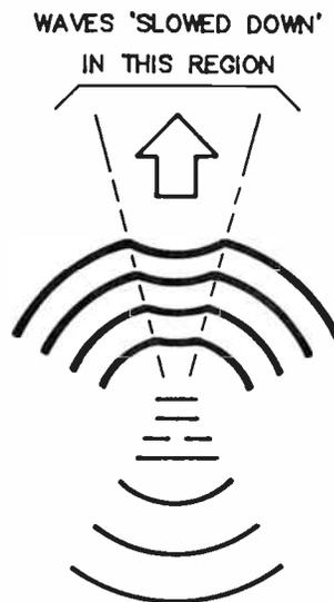
Figure 2. Adding a structure on the side of the dipole opposite the reflector slows down the waves and narrows the beam in this direction.
