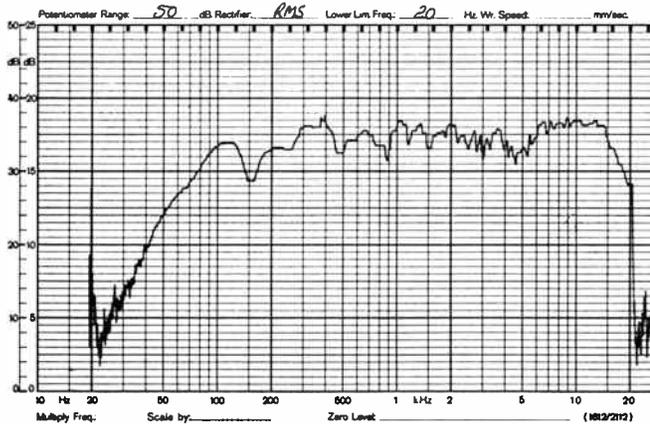
Figure 8. Frequency response of the KEF C10 speaker, measured on-axis.
