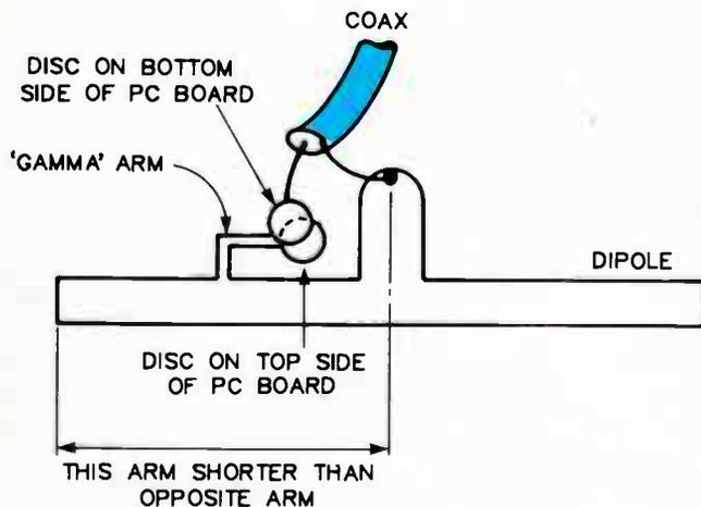
Figure 6. General arrangement of the driven element employed in this project. The effect of the gamma match on the operation of the dipole is compensated for by shortening that side of the dipole.
