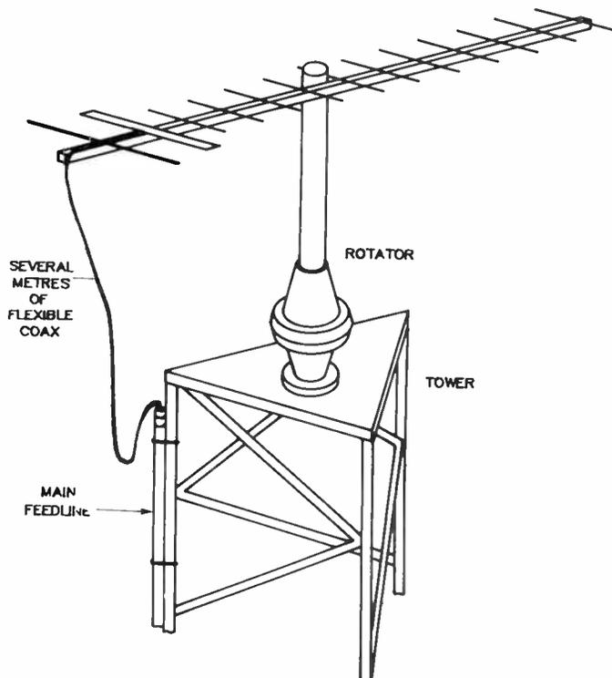
**Figure 11.** Several metres of flexible coax must be run between the antenna connection and the main feedline, sufficient to allow rotation without straining the cable.
