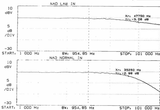
Figure 1 (above) & 2 (below). NAD 2200 power amp frequency responses for the 'lab' and 'normal' inputs.
