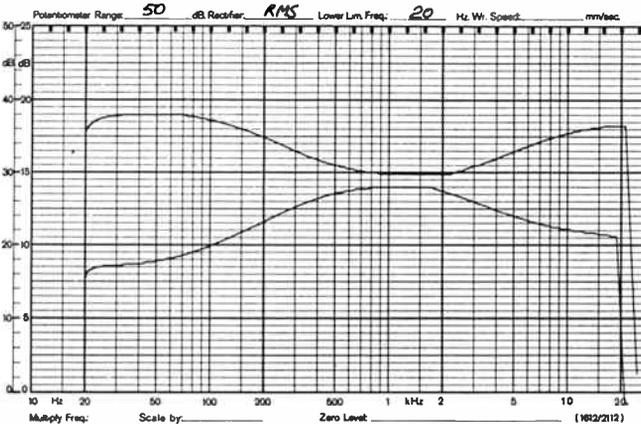
Figure 5. Response of the tone controls on the NAD 1155 preamp.
