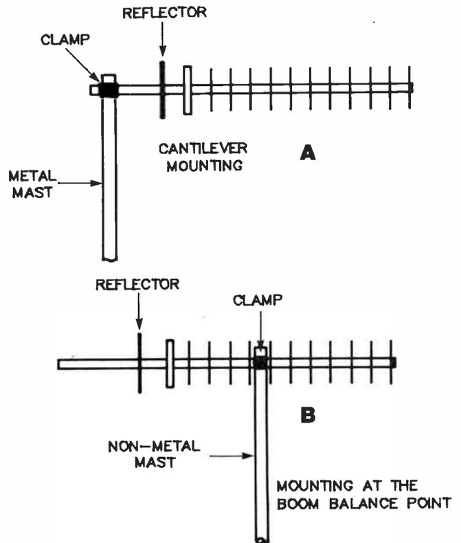
Figure 8. Vertical polarisation mounting arrangement — (a) shows cantilever mounting where a metal mast is employed, (b) shows mounting at the boom balance point, but here a non-metallic mast must be used.
