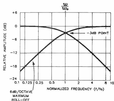
N.B:  $V_{\text{OUTH}}$  and  $V_{\text{OUTL}}$  are in phase quadrature (i.e.: 90° out of phase) which leads to a skewed polar response in the vertical plane in front of the loudspeaker.
