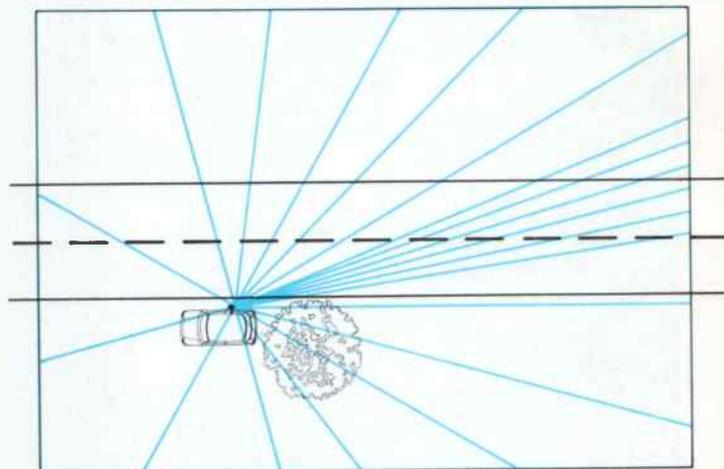
Figure 1. The down-the-road radar beam. The density of lines represents 'strength' of the beam. Remember that the beam is theoretically infinite in length in all directions.
