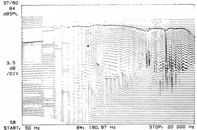
Figure 16. Impulse response of the C10 speaker shows only minor irregularities around 4 kHz and 7.35 kHz.
