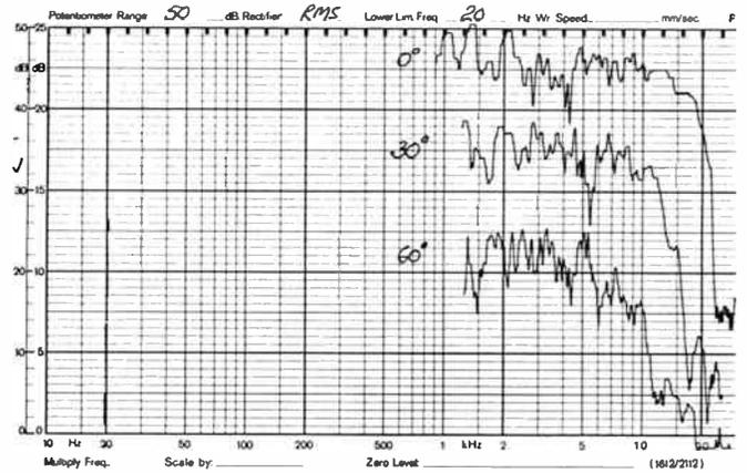
Figure 10. High frequency response of the C10 speaker at three different angles in the horizontal plane. Note — each trace has been separated by 10 dB for clarity. The top trace is on-axis.
