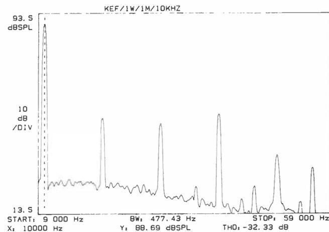
Figure 15. The 10 kHz/1 watt THD of the C10 is also very good, being a little better than -32 dB.
