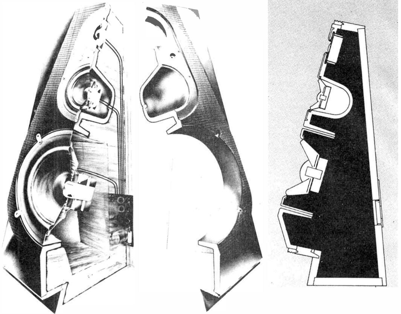
Figure 4. Showing the asymmetric cabinet design of the new Jamo Digital Monitor CBR series speakers. No sides are parallel so as to reduce cabinet internal resonances. The front panel is angled to align the acoustic centres of the drivers to obtain 'time coherent' sound radiation. The photograph shows a cutaway view of the CBR 200.
