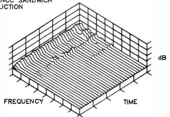
Figure 3. Comparison of the time decay spectral response to a pulse applied to 20 mm chipboard (upper graph) and Jamo's NCC sandwich construction (lower graph). Both materials were 'hit' with a pulse containing all frequencies between 20 Hz and 7 kHz. These vibration measurements show the damping characteristics of the two materials. The less 'landscape' there is, the fewer resonances there are, and hence the better the damping.
