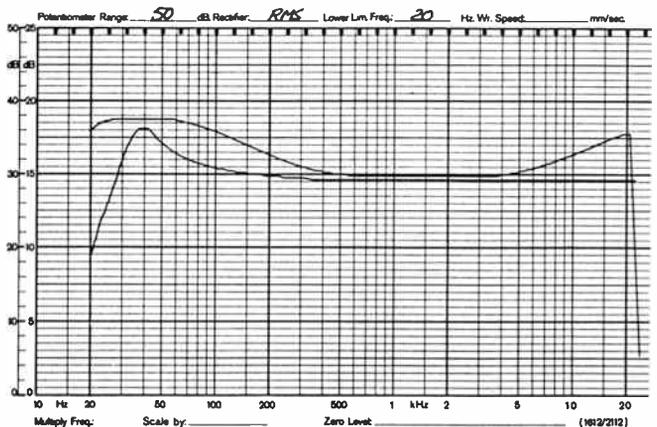
Figure 6. Superimposed curves of the loudness (upper trace) and bass eq (lower trace) switches of the NAD 1155.
