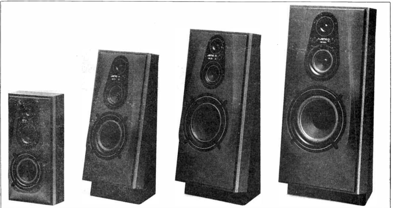
The resulting baffle construction comprises two layers of vacuum-formed polystyrene with the concrete-like material injection moulded between to form a sandwich 25 mm thick. The outer polystyrene skin of the baffle incorporates a moulded anti-diffraction pattern to preserve the stereo image at the upper end of the audio range. See Figure 2.
