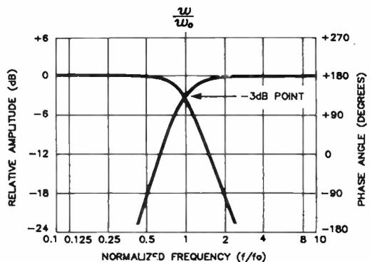
N.B:  $V_{OUTL}$  and  $V_{OUTH}$  are in phase quadrature again (as in the 1st-filter).
