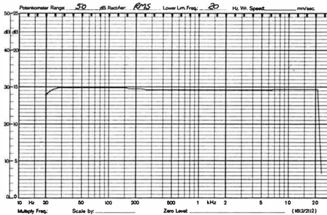
Figure 3. Overall frequency response of the NAD 1155/2200 combination.
