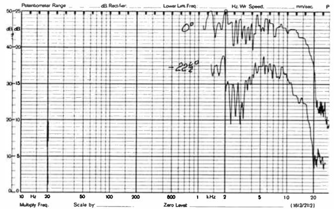
Figure 11. Vertical plane high frequency response of the C10 speaker on-axis (upper trace) and at 22.5 degrees below the horizontal. (Traces separated 10 dB for clarity). Note the phase cancellation around the crossover frequency on the lower trace.
