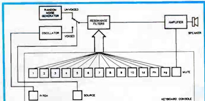
Figure 2. The first electronic speech synthesiser, built by Homer Dudley's team at Bell Labs in the US in 1939. Dubbed the "Voder", it was 'played' by keys and a pitch pedal, producing quite good results when used by a skilled operator. This was the forerunner to the modern-day "Vocoder" occasionally used in music recording.
