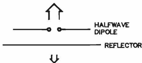
Figure 1. The dipole with parasitic reflector was the forerunner to the Yagi. There is more radiation in the direction away from the reflector and less in the direction of the reflector.
