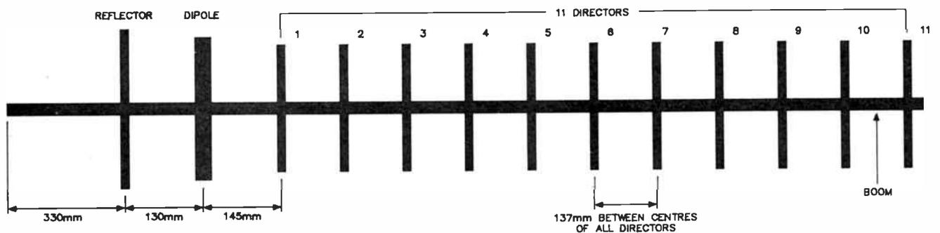
Figure 4. General assembly details and dimensions.
