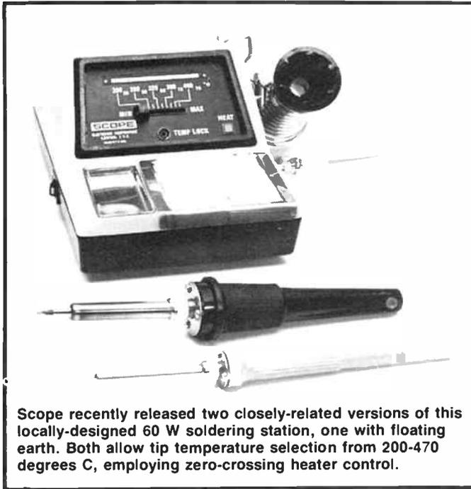
Scope recently released two closely-related versions of this locally-designed 60 W soldering station, one with floating earth. Both allow tip temperature selection from 200-470 degrees C, employing zero-crossing heater control.
