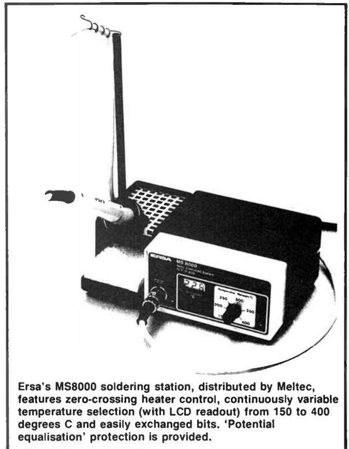
Ersa's MS8000 soldering station, distributed by Meltec, features zero-crossing heater control, continuously variable temperature selection (with LCD readout) from 150 to 400 degrees C and easily exchanged bits. 'Potential equalisation' protection is provided.
