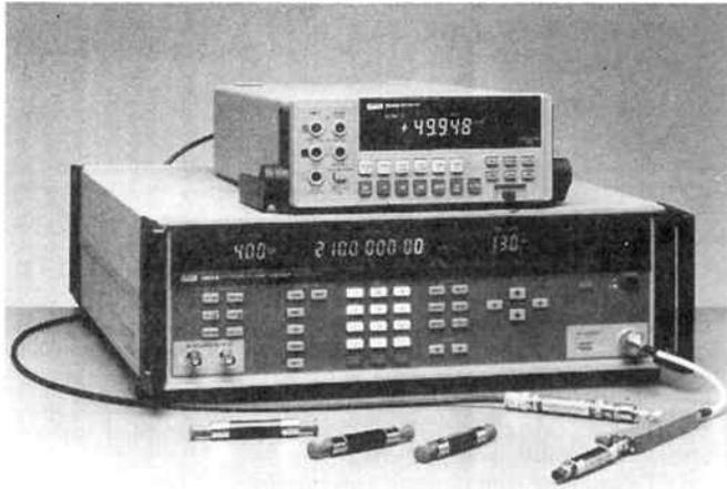
**E**lmeasco Instruments has introduced the Fluke 6062A Synthesized Frequency Generator, with signal generation capabilities from 100 kHz to 2.1 GHz. In addition, it incorporates a high-performance pulse modulator.
