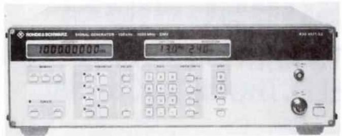
A typical example of today's professional instruments, this RF signal generator from Rhode & Schwarz covers the range from 0.1 to 1000 MHz and provides AM, FM and pulse modulation as well as a digital readout of frequency, amplitude and modulation. Rhode & Schwarz Australia are available on (02)267 2622.
