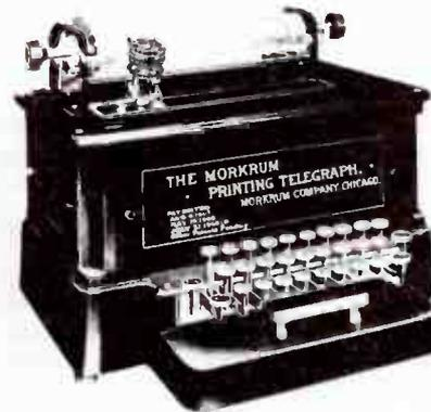
**This illustration shows a very early example of the teleprinter or "printing telegraph" made by the Morkrum Company of the USA. Despite becoming more streamlined, modern machines still use the same basic method of operation.**
