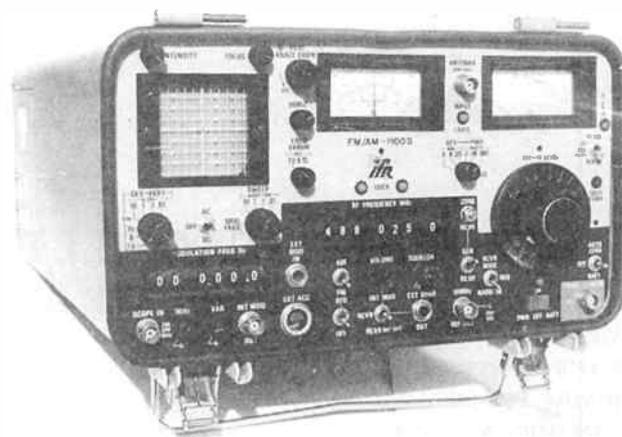
**This multi-function instrument from IFR will be familiar to many radio technicians. The instrument combines such features as a signal generator, monitor receiver and deviation meter with a portable spectrum analyser. The IFR range is available from Vicom Australia. (03)690 9399.**
