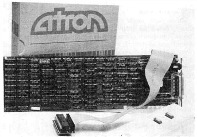
**Here's something different! This board, the PC Probe by Atron, is a real-time hardware assisted software debugging tool for C, Pascal, Fortran and Macro Assembler. Available from Macro Dynamics (03)220 7260.**
