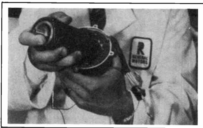
The "magnaquench" dc motor develops two horsepower (1.5 kW) continuously at 4000 rpm but weighs less than 4 kg! It has a stationary outside winding and no brushes. It was connected to the left rear wheel via a 4:1 chain drive.
