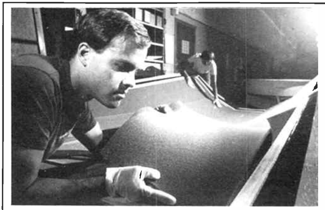
The body of Sunraycer was made up of a composite material comprising a sandwich of Kevlar-Nomex-Kevlar, which was strong, rigid and very light (3 oz per square foot).
