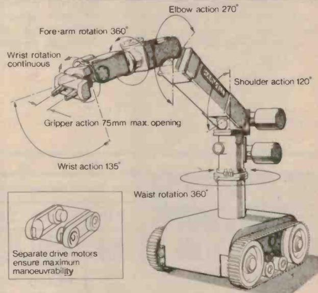
Fig. 5. ROMAN, a recent Harwell mobile, is made for use in hazardous industrial situations. It is electrically powered using cable control.
