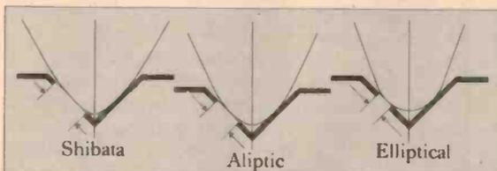
It is basically elliptical (.0003" x .0007"), but its bottom radius has been modified to extend the vertical bearing surface on the groove wall by 100%.
