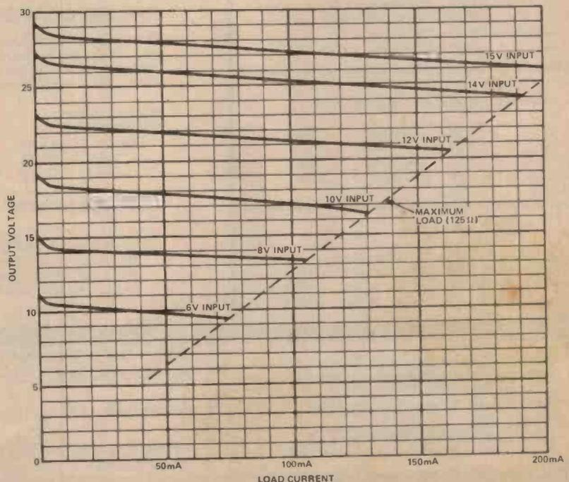
Fig. 5. Graph showing the relationship between the output voltage and load current for various input voltages.
