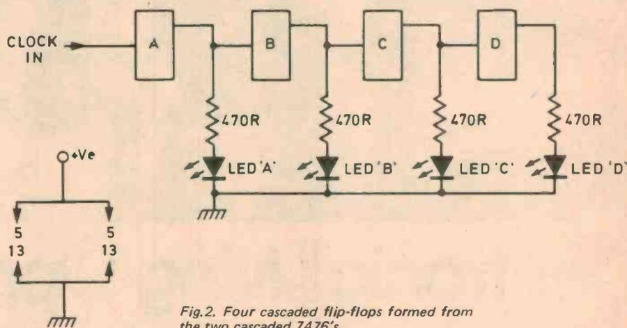
Fig. 2. Four cascaded flip-flops formed from the two cascaded 7476's.
