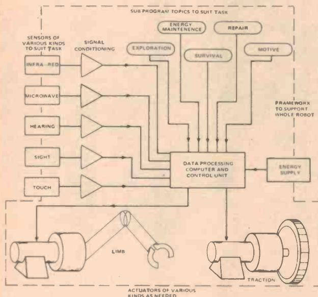
Fig. 2. Robot systems are made up from sensors, actuators and data processing systems operating together to satisfy a number of operational requirements.
