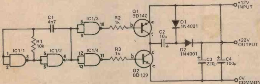
Fig. 4. The circuit diagram of the +22V version.
