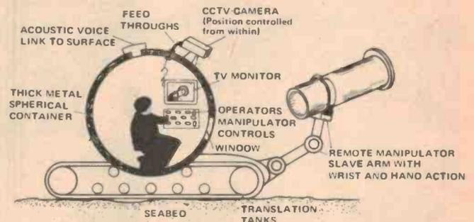
Fig. 3. Underwater a robot manipulator provides an operator with an effective ecoskin and increased ability to do work.
