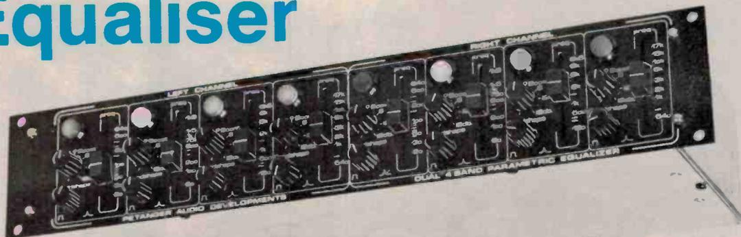
The Petanger Dual 4 band Parametric is a state of the art stereo equalizer consisting of 4 independent filter sections in each channel. Each filter is capable of continuous adjustment of amplitude, frequency and bandwidth.
