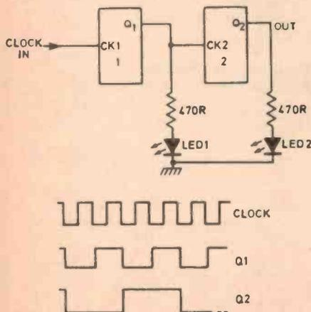
Fig. 1. Cascading 7476 flip-flops.
