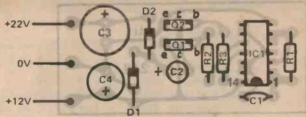
Fig. 2. The component overlay of the +22V version.
