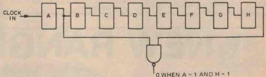
Fig. 7. A 'ripple counter'. This type of counter can suffer from 'race hazards'.
