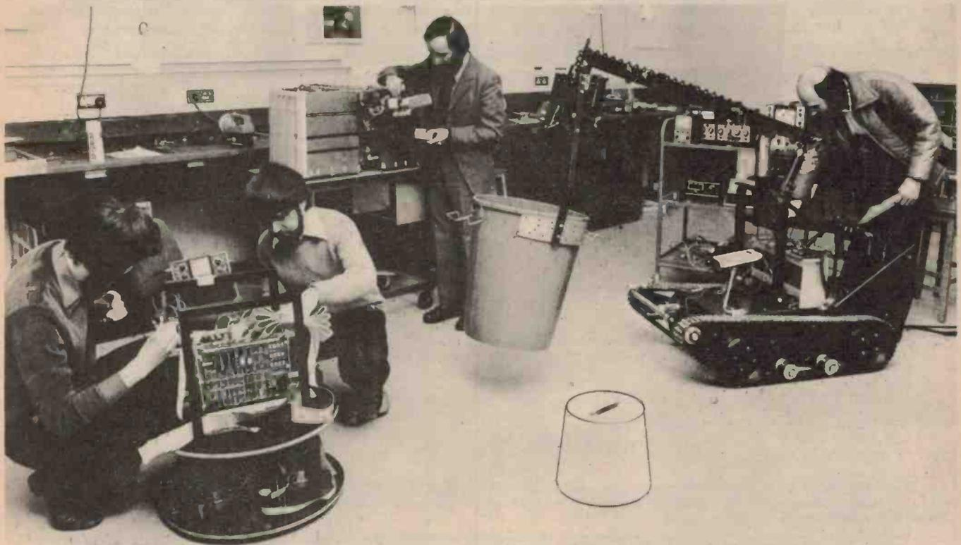
Fig. 1. Projects of the Warwick University Robot Laboratory. Project on the left uses an inboard microprocessor. At the rear is a hand-like short arm manipulator. The tracked vehicle is originally
