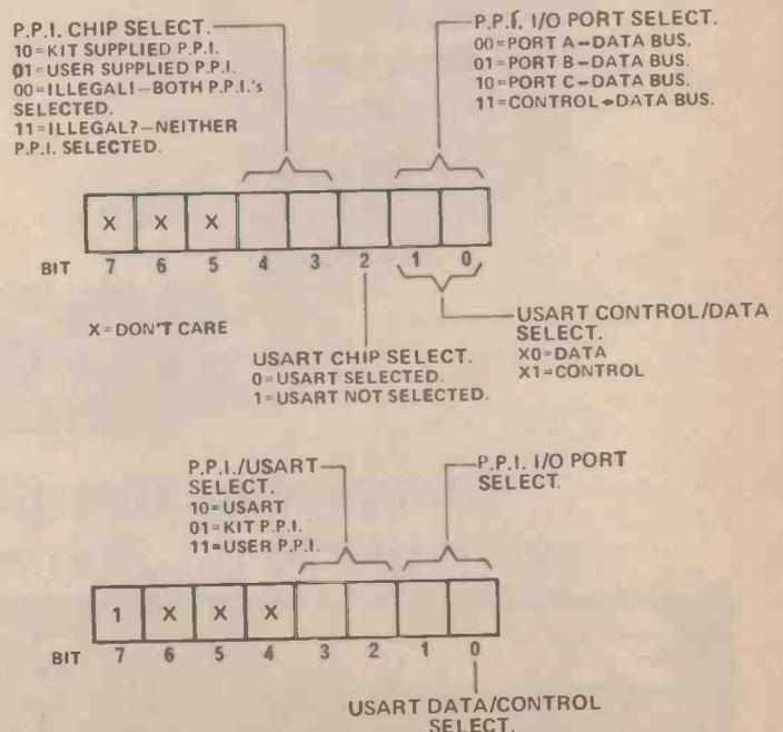
Fig. 6. SDK-80 combined PPI and USART device code format.
