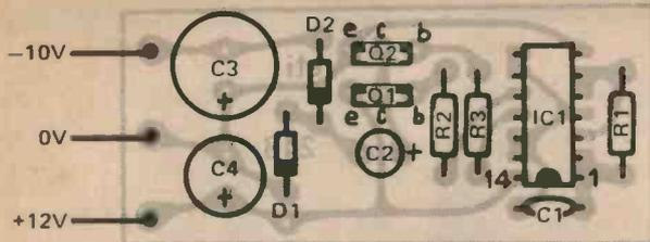
Fig. 1. The component overlay of the -10V version.
