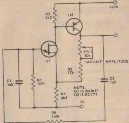
for sine wave outputs of 0.01 Hz. This capacitor is available in polycarbonate. The amplitude of the output can be adjusted by RV1 to give low harmonic distortion and to be about 10V peak to peak. As expected, with this Wien bridge circuit, frequency stability is good with changes in both supply voltage and temperature.
