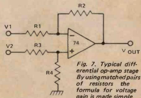
Fig. 7. Typical differential op-amp stage. By using matched pairs of resistors the formula for voltage gain is made simple.
