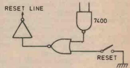
Fig. 6. Using a push-button reset with the circuit of Fig. 5. This could be accomplished in several other ways.
