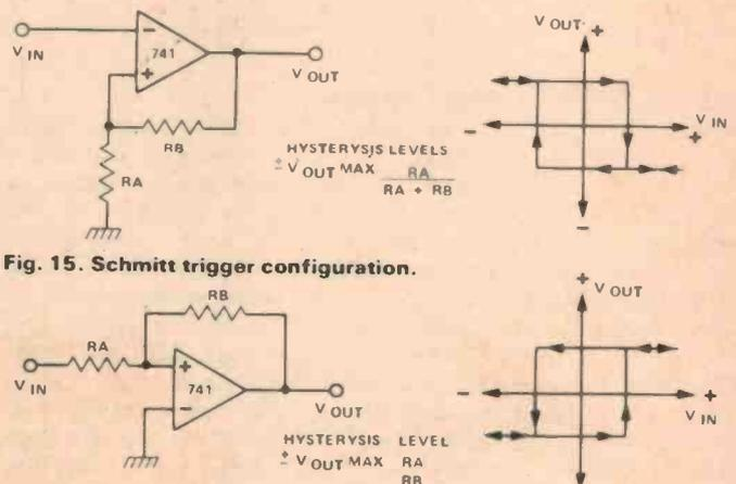
Fig. 15. Schmitt trigger configuration.
