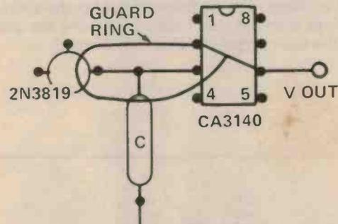
circuit to keep the leakage currents to a minimum. Also, to stop surface leakage a simple PCB trick can be used, that of making a guard ring around the sensitive components.
