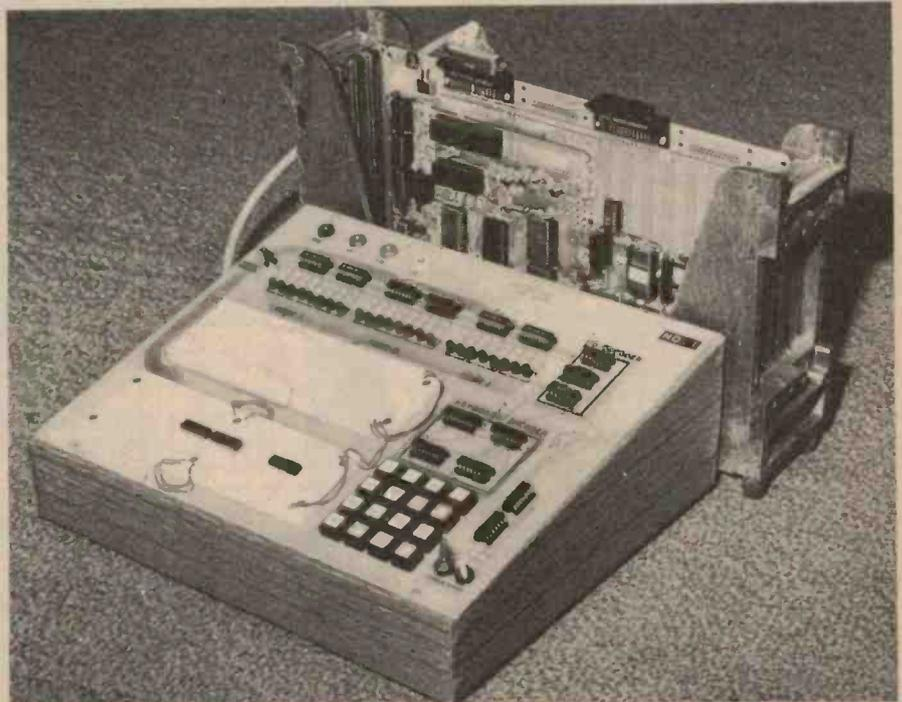
Fig.1. A prototype of the educational/prototyping microcomputer. The SKD-80 (at rear) is connected to the MMD-1 educational interface via the 43 pin P-1 edge connector and the 25 pin J-1 edge connector.
