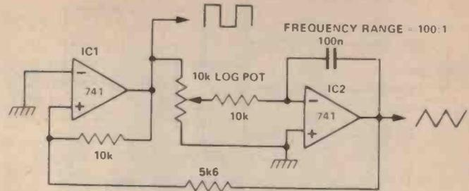
circuit is the basis of most function generators. By bending the triangle it is possible to synthesise an approximation to a sinewave. With a bit more electronics it is also possible to make the oscillator voltage controlled.
