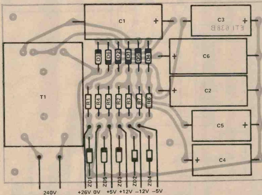
Fig. 2. The component overlay of the power supply.
