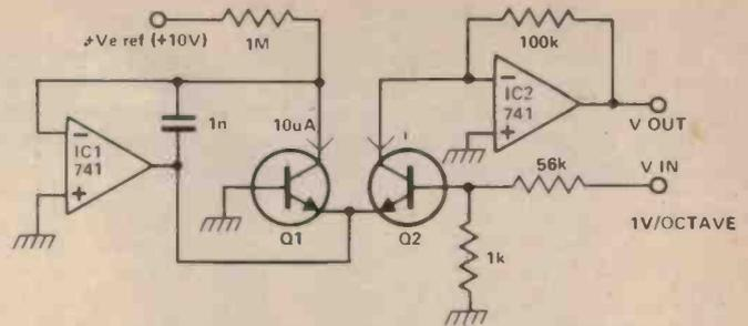
has a high temperature coefficient ( $-1.9 \text{ mV}/^\circ\text{C}$ ) and so the reason for using a matched pair is to use the first transistor, Q1, to provide temperature compensation for the second.
