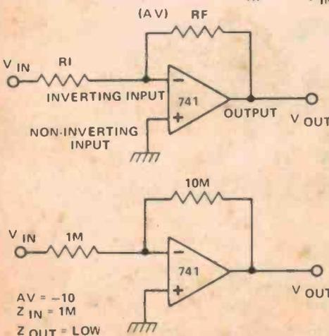
Figs 1 and 2 show (upper) the basic inverting op-amp stage. Gain is given by the ratio of resistors  $R_F/R_I$ , input impedance is simply  $R_I$ , while the output impedance is more complicated (see text). Fig. 2 (lower) shows a stage with a gain of 10 and an input impedance of 1 M.
