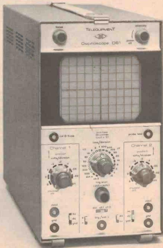
plete trace each time. In the third method the beam draws both traces in one sweep by alternating very quickly between traces. In this "chopped" mode the beam may draw say .1 mm of the top trace, then .1 mm of the bottom one, then back to the top, etc.
