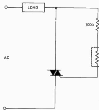
**Fig. 8. Photo-cell coupling provides electrical isolation.**
