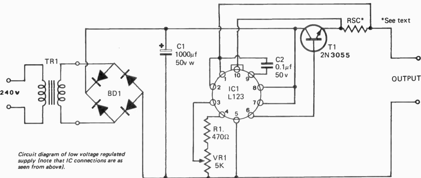
Circuit diagram of low voltage regulated supply (note that IC connections are as seen from above).
