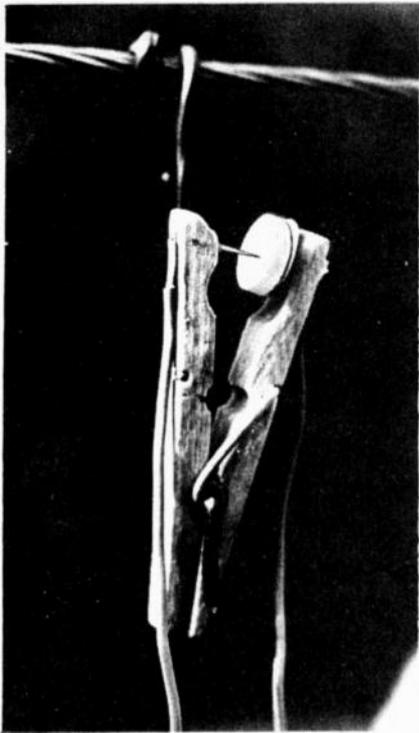
Vertically suspended hygrosopic transducer features disposable actuating element.
