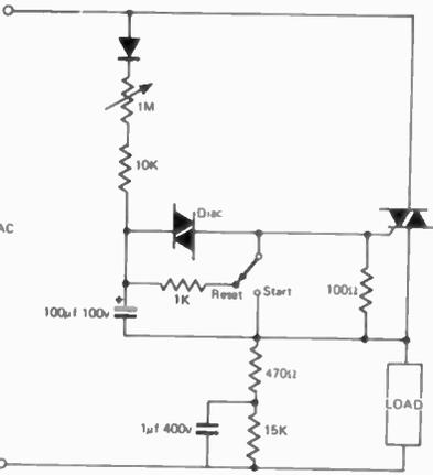
**Fig. 12. Time delay circuit — action similar to Fig. 11.**
