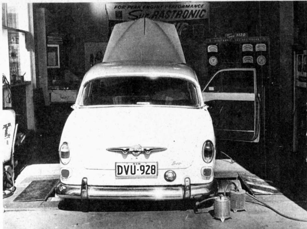
Volvo's power output is checked by chassis dynamometer. Units near exhaust pipe remove water vapour from gas sample.
