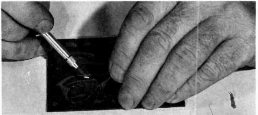
Fig. 10. Remove remaining film from the board.
