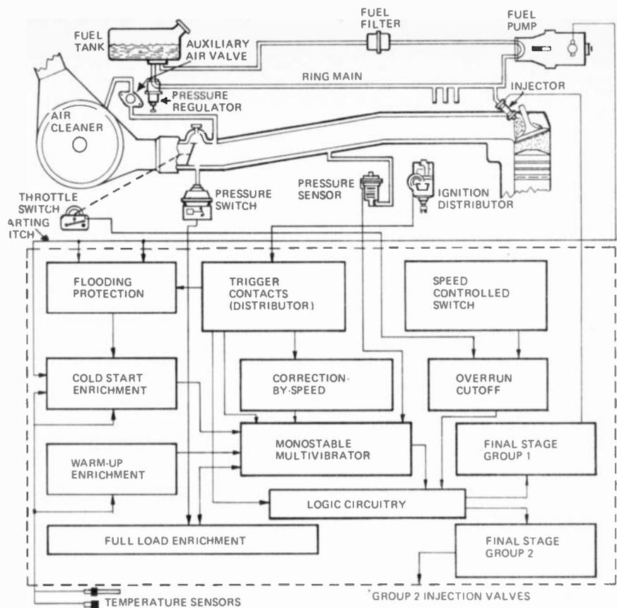
Fig. 1. Schematic drawing of fuel injector system.
