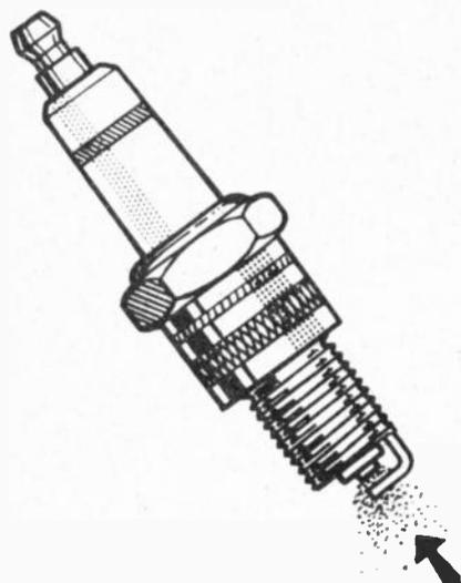
Fig. 3. Hot centre electrode of spark plug emits electron cloud which assists spark to jump to positive (colder) earth electrode.
