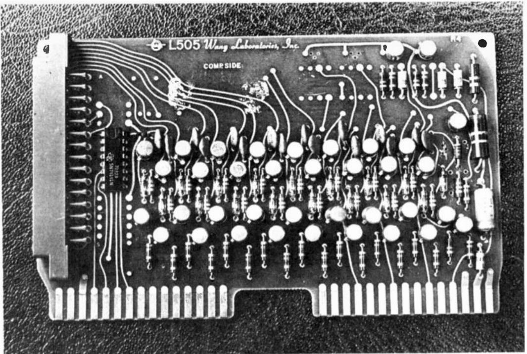
Plug-in circuit boards simplify maintenance and fault-finding.
