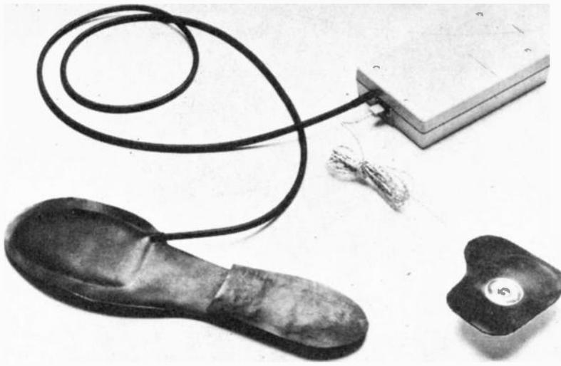
Complete kit consists of a rubber inner sole with small air chamber (left), connected by a tube to a pneumatic switch in a pulse generator (top right) which in turn is connected to an electrode (bottom right).
