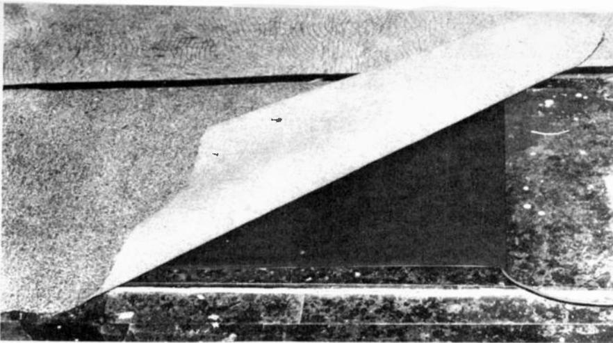
Fig. 13. Pressure mat installed under carpet or rug in strategic passage.
