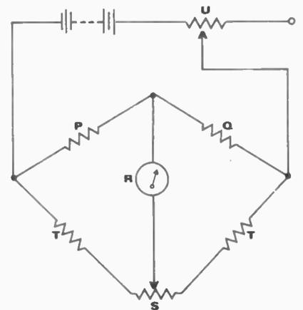
Electrical Circuit of thermal conductivity Exhaust Gas Analyser: (P) gas cell, (Q) air cell, (R) air-fuel ratio meter, (S) air-set calibration, (T) fixed precision resistors. (U) bridge voltage calibrator. Fig. 14.
