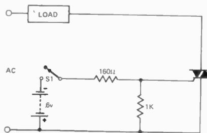
Fig. 2. Triac triggered by external dc voltage.
