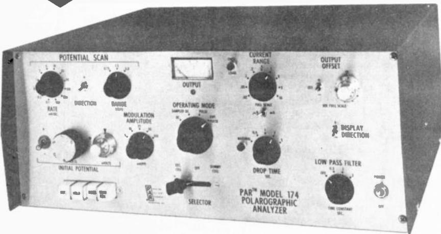
The instrument incorporates a  $\pm 80$  volt potentiostat for 3 electrode operation and has current sensitivities as high as 20 nanoamps full scale. It also features variable pulse amplitude for differential pulse polarography, and provides scan rates from 0.1 to 500 millivolts per second. Plug-in circuit boards permit quick, easy service.
