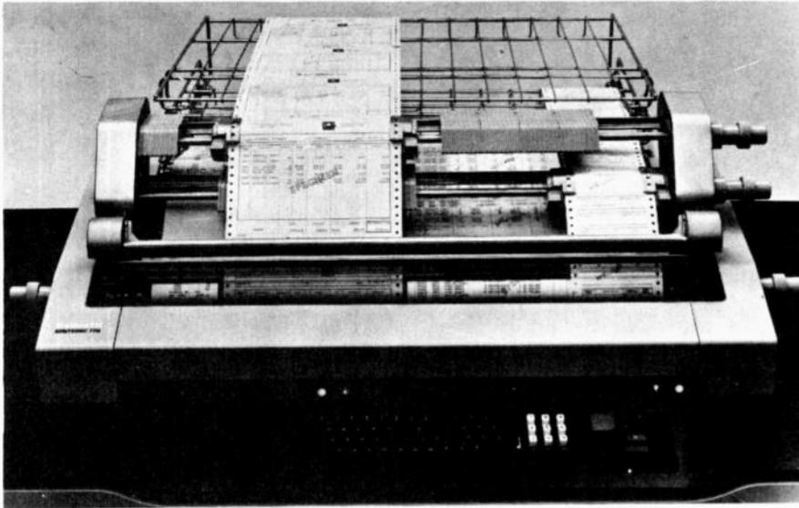
**T**HE OLIVETTI Auditronic 770 is a visible record computer designed to fill the gap between sophisticated accounting machines and large-scale computers.
