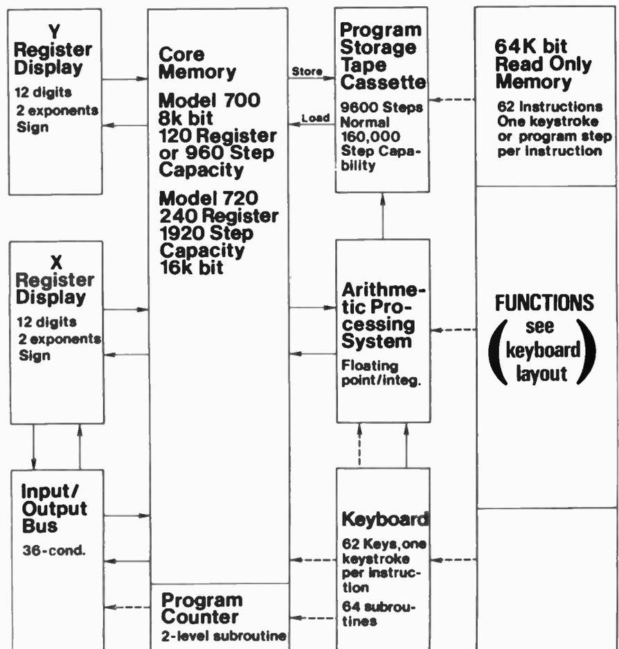
Block schematic diagram of Wang 700 series calculators.
