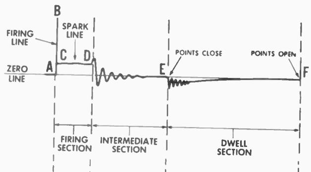
**FIG. 1 — BASIC SECONDARY WAVEFORM**
