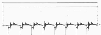
Fig. 4. Reversed coil polarity — complete pattern is inverted.
