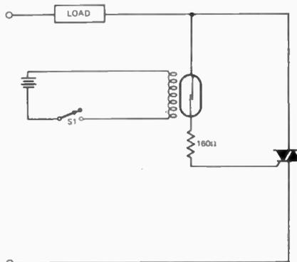
Fig. 6. Reed relay can be electrically operated to provide electrical isolation.
