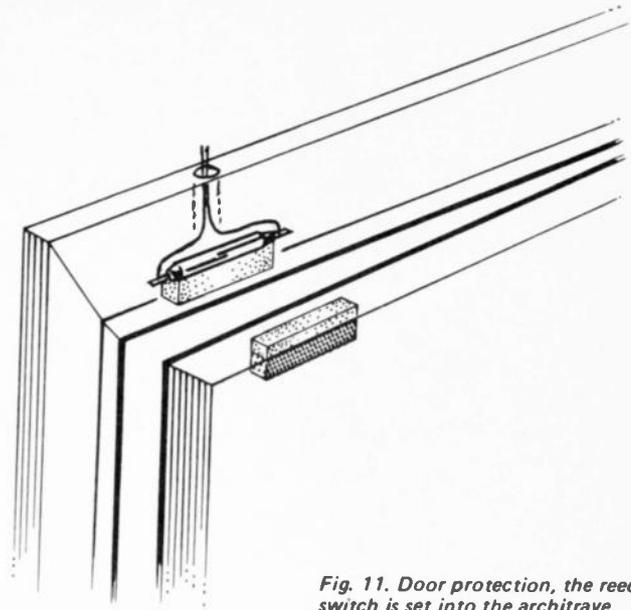
Fig. 11. Door protection, the reed switch is set into the architrave.
