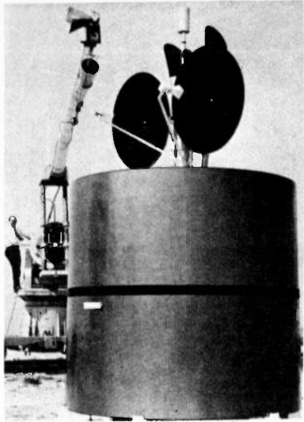
*Antenna test — A full-scale model of the huge Intelsat-IV communications satellite looms in foreground while an engineer conducts an antenna range test to verify radio frequency patterns of the horn antenna (mounted on boom).*
