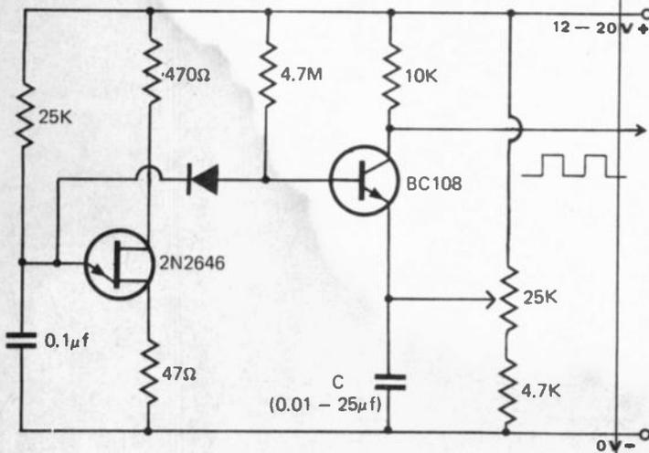
A variable duty cycle squarewave can be obtained from this unijunction circuit. The light loading imposed on the emitter timing circuit preserves frequency stability.
