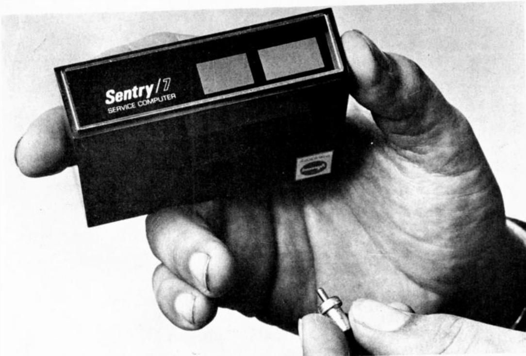
Ingeniously simple unit from Plessey monitors engine usage and indicates when to change oil.
