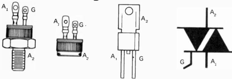
Fig. 1. Construction and electrical connections of typical Triacs.
