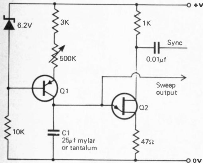
This circuit provides a linear time-base with a sweep time adjustable from a few milliseconds to over one minute.
