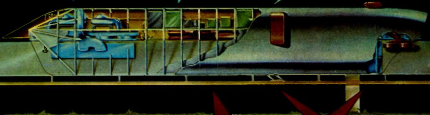
The experimental tracked air cushion vehicle, which Tracked Hovercraft Limited aims to have under full-scale test this year is shown cut-away to indicate the amidships positioning of the 6,500 lb thrust single-sided linear motor used for propulsion, and the hoverpads used for support and guidance. The vehicle is designed to reach 300 mph, towards the end of 1972, when the test track at Earith, in England is extended to eight miles in length.
