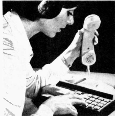
A new telephone set recently developed by Germany's Siemens Industries can also double as a data terminal.
