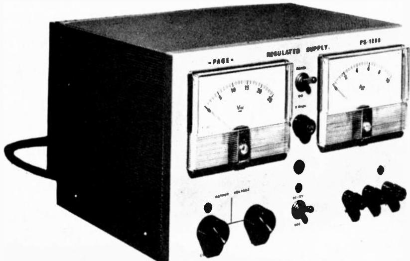
This regulated power supply, designed and made in Australia, provides outputs adjustable from 9 to 16 volts at currents of up to 15 amps.
