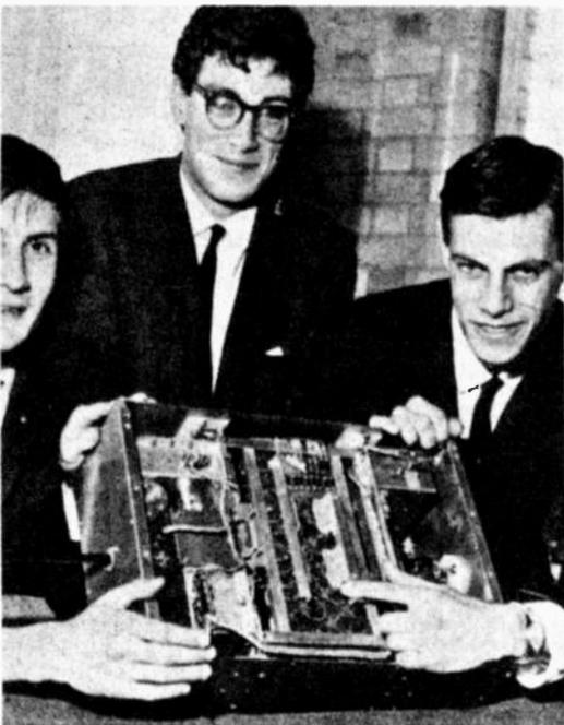
*This is a look inside of the fifth and most recent satellite to be launched successfully in the Oscar series. Designed and constructed in Australia by students of Melbourne University (three of whom are in our photograph), this was the first amateur satellite to be ground-controlled. Hundreds of amateur stations throughout the world used the satellite's 10- and 2-metre telemetry-beacon transmissions for tracking, propagation and other scientific investigations during early 1970.*
