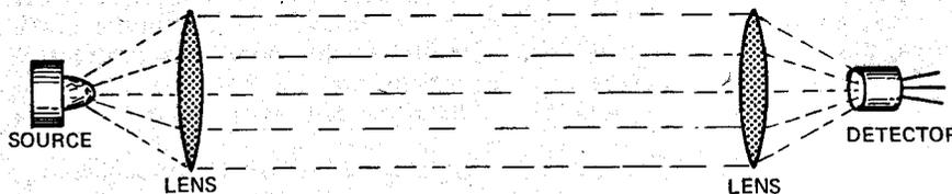
Fig. 1. A basic opto-electronic system.
