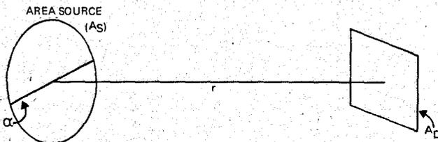
Fig. 5. Area source geometry.
