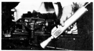
A simple hand held instrument for rapid detection of leaks. Designed to meet British Ministry of Defence-Navy requirements
