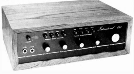
Simple, yet effective unit has SQ plus ambience decoding - and produces 15 watts per channel.
