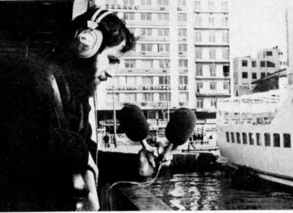
Recording the departure of a ship from Piraeus Harbour (Greece). Equipment used to make this stereo recording includes Neumann KM76 condensor microphones and windshields. Senheisser headphones are being used to monitor the output from the Stellavox SP7 recorder.
