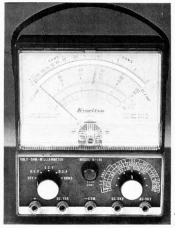
Typical high quality multimeter, note the 'ohms' scale in which zero is at right hand end. Meters that indicate the measurement by a scale and moving pointer are known generically as 'analogue' instruments.
