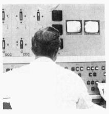
Two Philips circuit television cameras are vital for the efficient operation of an automatic control system in the Ultimo (Sydney) plant of Dairy Farmers Co-operative Ltd. They are used to check valve settings and flow lines.
