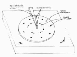
Fig, 4, Electro-mechanical rythm generator.
