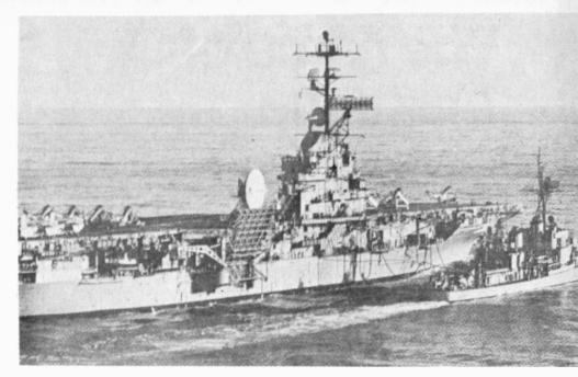
Fig. 14. Communication links sending measurement and control data are known as telemetry systems. In the picture above the round white dish antenna receives data from television cameras in space.
