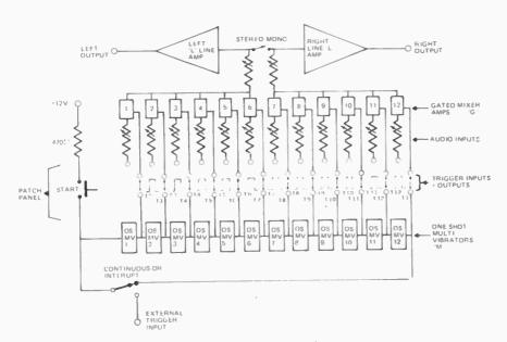
Fig. 1. Twelve channel switching mixer (designed by Ehle).
