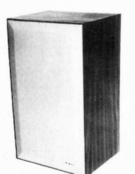
DRIVERS 12" Twin Cone Woofer. 2½" Super Tweeter. FREQUENCY RESPONSE 37 Hz to 20,000 Hz. CROSSOVER FREQUENCIES 2500 Hz MINIMUM POWER REQUIREMENT 5 Watts RMS MAXIMUM POWER HANDLING 30 Watts RMS NOMINAL IMPEDANCE 8 Ohms COLORS AVAILABLE: RED, BLUE, BLACK, BROWN. TIMBER WALNUT FINISH SIZE 24 3/8" H x 14½" W x 12" D
