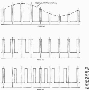
Fig. 13. Modulation of pulse carriers. (a) Pulse amplitude modulation PAM. (b) Pulse width modulation PWM. (c) Pulse position or pulse time modulation PPM or PTM. a total bandwidth of 12 000 Hz (plus channel separation).
