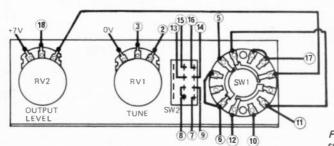
Fig. 4. Wiring diagram for switches potentiometres.
