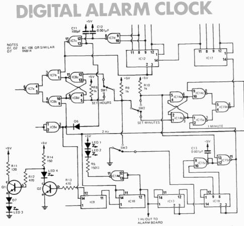
Fig. 3. Modified circuit diagram incorporating AM/PM indication and improved time setting facilities. Part only of complete circuit shown.
