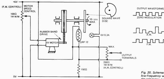
Fig. 20. Schematic layout of the mechanical low-frequency waveform generator used in the telemetry systems discussed.
