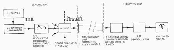
Fig. 18. Block schematic of pulse amplitude modulated communication link.
