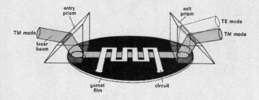
Path of a laser beam through the thin film switch
