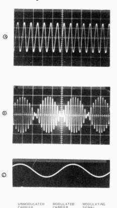
Fig. 10. In amplitude modulation, the amplitude of the a.c. carrier signal is varied, the frequency remaining the same. modulate an ac signal — it needs a special generator to produce the carrier in the first place and special circuits to recover the signal when received.
