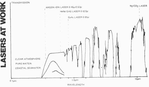
Fig. 9 Transmission of EM radiation.
