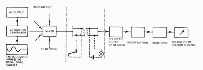
Fig. 19. Block schematic of a pulse frequency modulated link.
