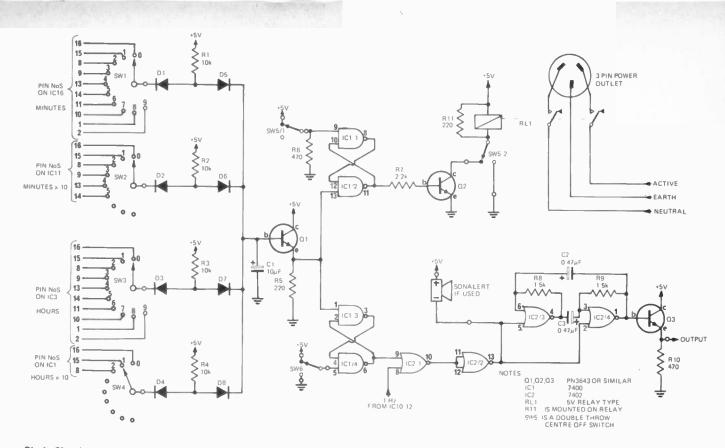
Fig.1. Circuit diagram of the complete alarm facility. Note that SW5 has three positions - Power Outlet On, Off, and Power Alarm On.
