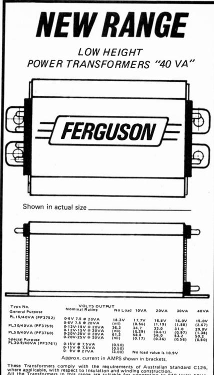
These Transformers comply with the requirements of Australian Standard C126, where applicable, with respect to insulation and winding construction. All the Transformers in this range are suitable for connecting to 240 Volts 50Hz, single phase supply. General purpose Transformers types PL15/40VA, PL30/40VA and PL50/40VA are provided with two identical secondary windings with a tap on each. This permits series or parallel operation.
