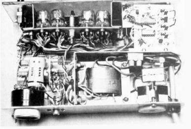
Rear of the clock showing Sonalert, oscillator output and set/run switch on the left and power outlet socket on the right.
