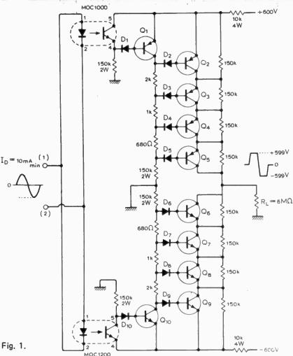
all the transistors Q2 to Q5 conduct and the output swings positive by 600 V minus  $V_{\rm SAT}$  for transistors Q2 to Q5.
