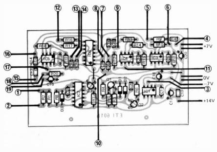
◀ Fig. 2. Component overlay of VCF.
