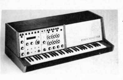
Fig. 13. (LEFT) EMS' sequencer has inbuilt digital memory bank.
