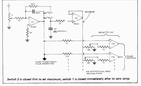
Fig. 6. Experimental circuit for rythm generator having 'live performance' control.
