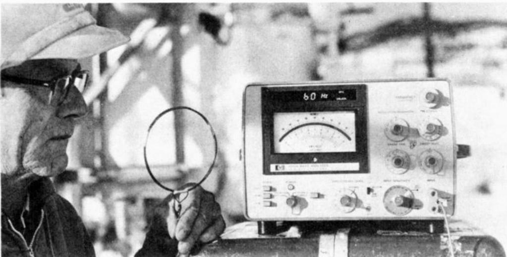
Accurate single-frequency measurements are fast and easy to make with this new Hewlett-Packard Model 3581A Wave Analyser. A built-in counter displays the tuned frequency unambiguously with 1 Hz
